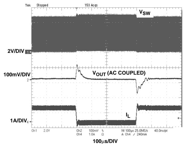
FIGURE 22. LOAD TRANSIENT TEST (MODE = GND,
