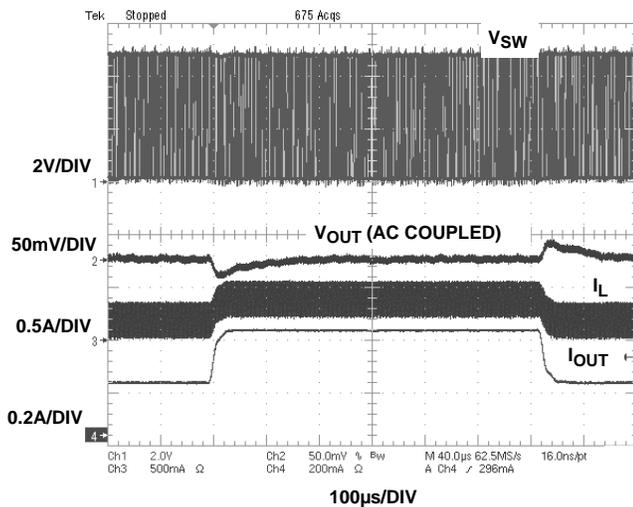
FIGURE 21. LOAD TRANSIENT TEST (MODE =  $V_{IN}$  = 5V;
