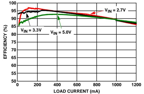
FIGURE 2. EFFICIENCY vs LOAD CURRENT ( $V_{OUT} = 2.5V$ )
