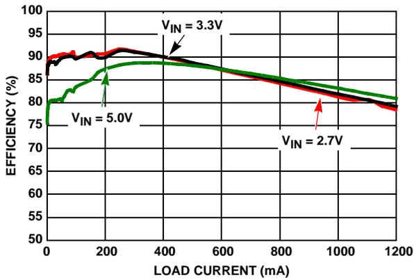
FIGURE 3. EFFICIENCY vs LOAD CURRENT ( $V_{OUT} = 1.8V$ )
