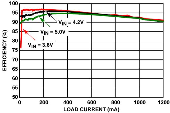
FIGURE 1. EFFICIENCY vs LOAD CURRENT ( $V_{OUT} = 3.3V$ )
