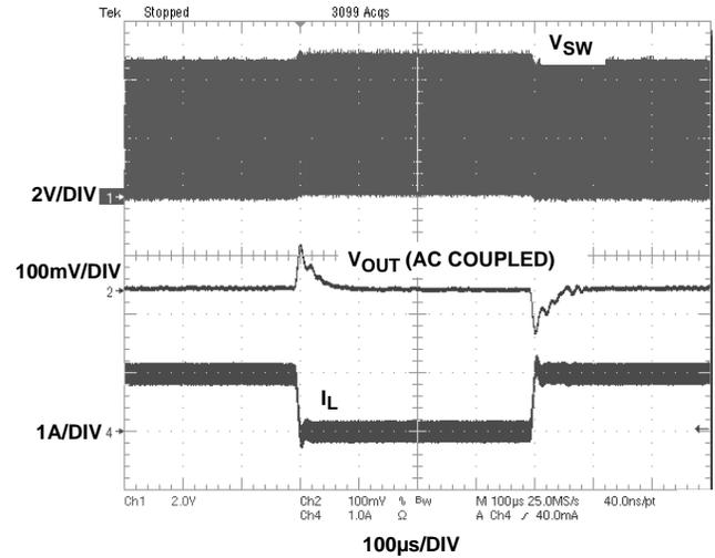
FIGURE 20. LOAD TRANSIENT TEST (MODE = GND,
