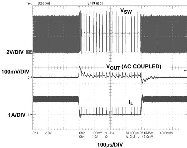
FIGURE 19. LOAD TRANSIENT TEST (MODE =  $V_{IN}$  = 5.0V;
