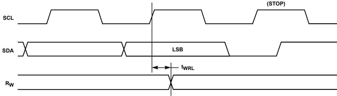
**Write Protect and Device Address Pins Timing**
