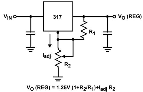
$$V_O (\text{REG}) = 1.25V (1 + R_2/R_1) + I_{\text{adj}} R_2$$
