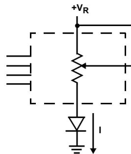
Two terminal Variable Resistor;
