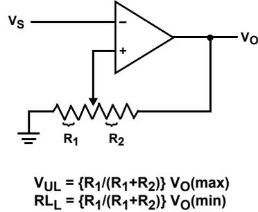
$$V_{UL} = \{R_1/(R_1 + R_2)\} V_O(\text{max})$$
