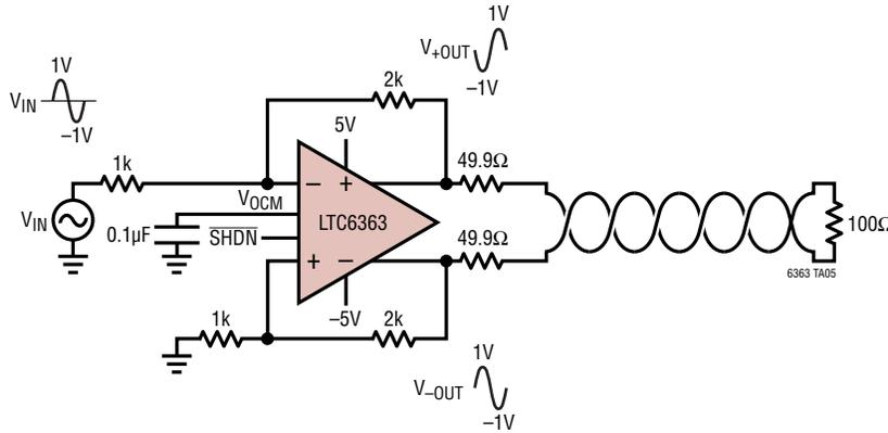
LTC6363 Used as Lowpass Filter/Driver with 10V<sub>p-p</sub> Singled-Ended Input, Driving a SAR ADC
