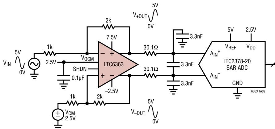
Differentially Driving an ADC with  $\Delta V_{IN} = 10V_{P-P}$  and Gain of  $A_V = 1$
