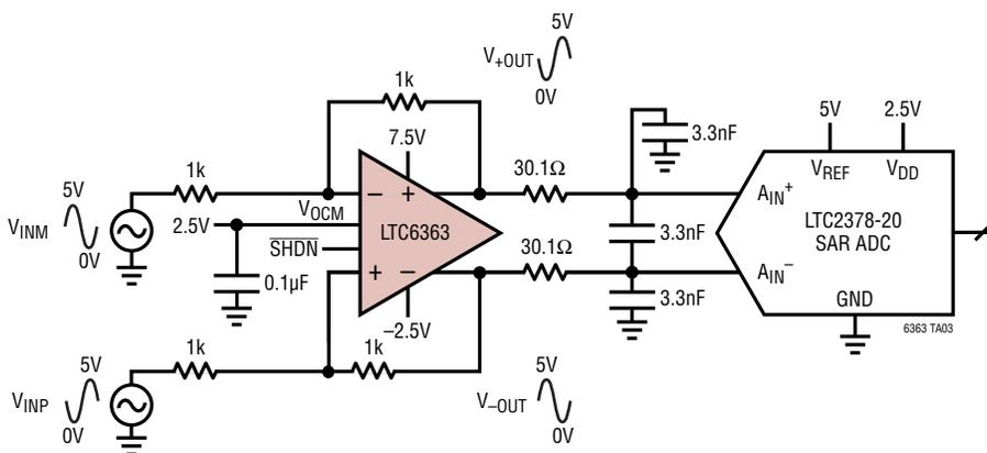
Differentially Driving a Pipeline ADC with  $A_V = 1$
