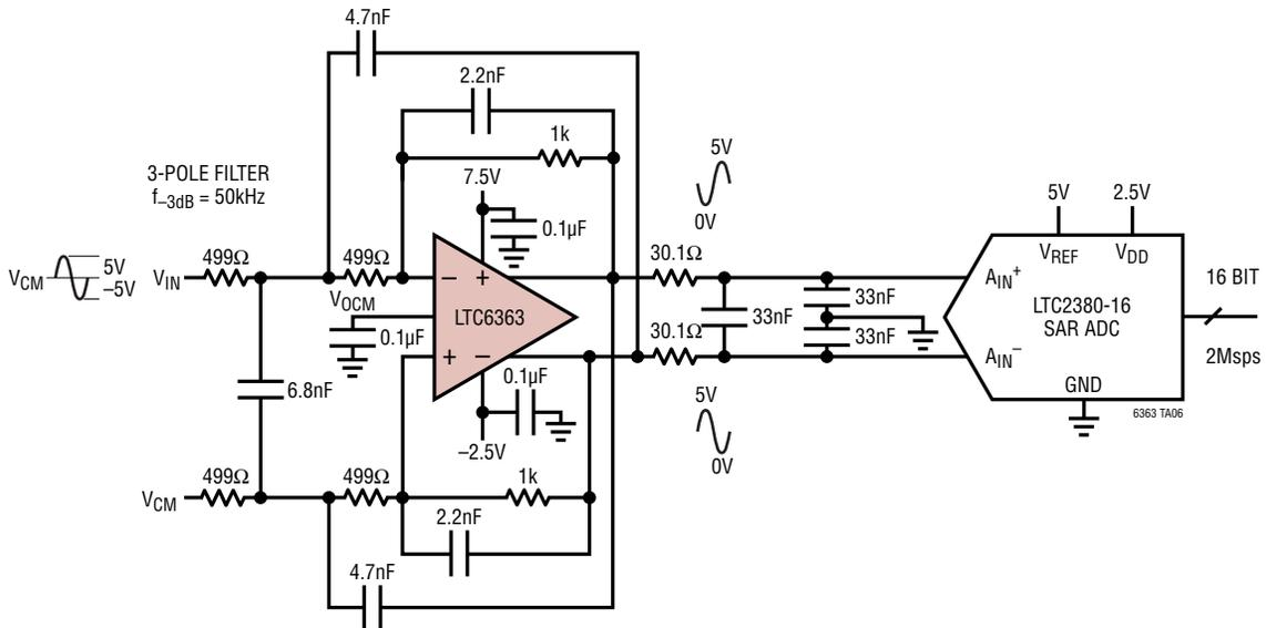
Differential  $A_V = 1/9$  Configuration Using an LT<sup>®</sup>5400 Quad-Matched Resistor Network
