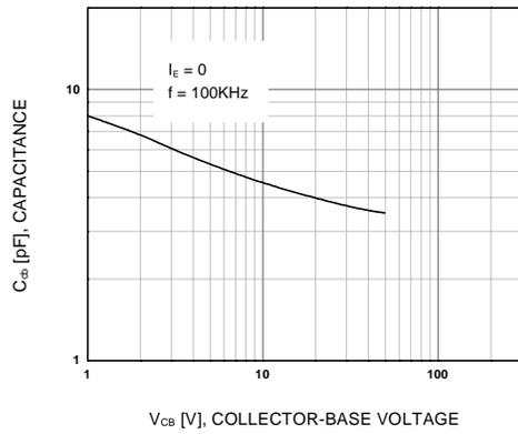
Figure 3. Collector-Base Capacitance
