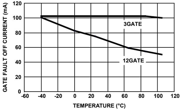
FIGURE 33. GATE FAULT OFF CURRENT (ABS) vs TEMPERATURE
