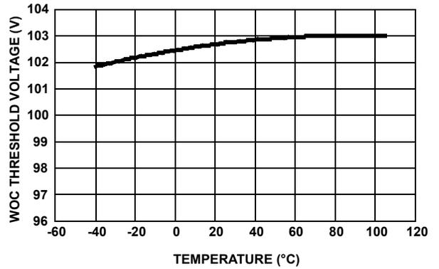
FIGURE 24. FAST TRIP THRESHOLD VOLTAGE vs TEMPERATURE
