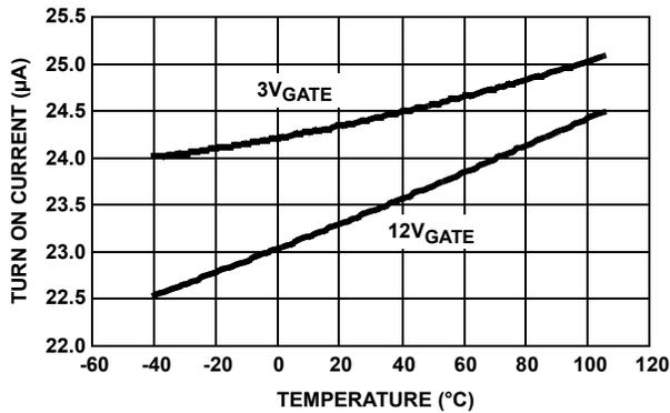
FIGURE 31. ISL6113 GATE TURN-ON CURRENT (ABS) vs TEMPERATURE
