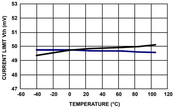
FIGURE 23. CURRENT LIMIT THRESHOLD VOLTAGE vs TEMPERATURE
