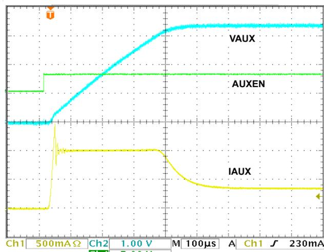
FIGURE 2. VAUX TURN-ON  $R_{LOAD} = 10\Omega$ ,  $C_{LOAD} = 100\mu F$
