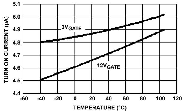
FIGURE 32. ISL6114 GATE TURN-ON CURRENT (ABS) vs TEMPERATURE
