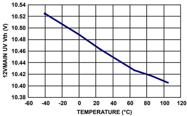
FIGURE 29. 12VMAIN POWER GOOD THRESHOLD VOLTAGE vs TEMPERATURE
