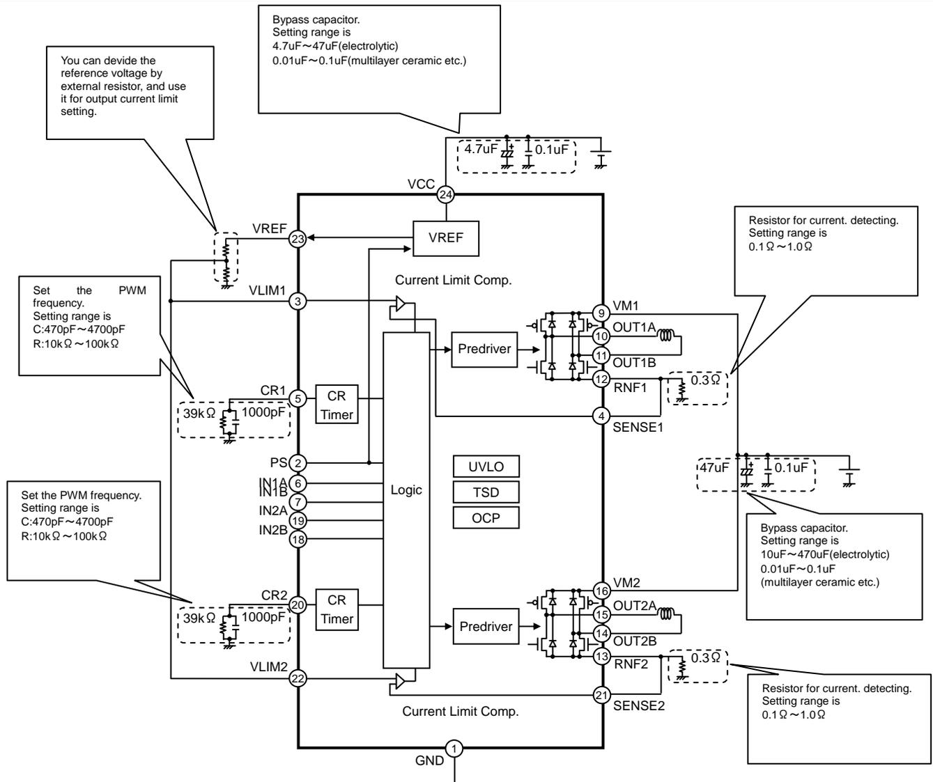
Fig.1 Block diagram & Application circuit diagram of BD6380EFV / BD6381EFV
