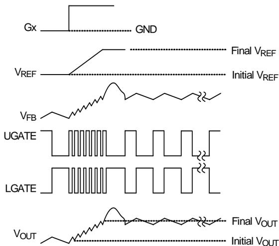
Figure 5. Output Voltage Up Transition with Overshooting
