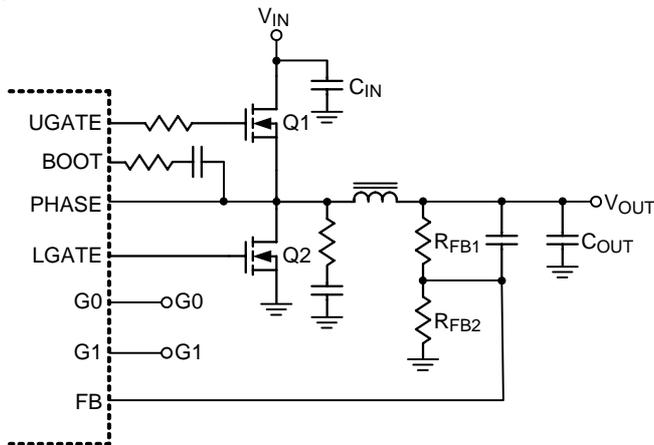
Figure 2. Setting V<sub>OUT</sub> with a Resistor-Divider
