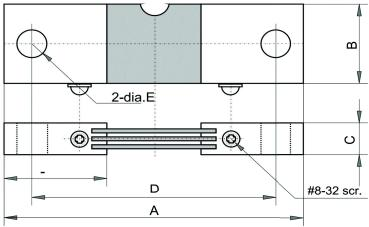
\*Dimension tolerances:  $\pm 0.381$ mm for hole diameteres. All other dimensions have a  $\pm 0.762$ mm tolerance
