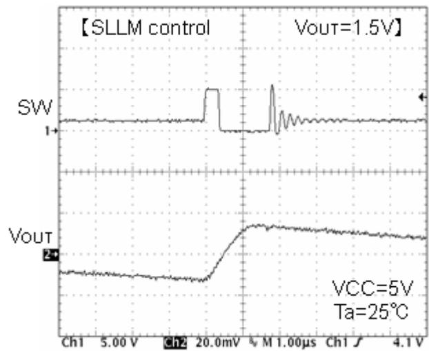
Fig.36 SW waveform I<sub>o</sub>=10mA
