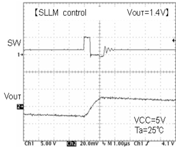
Fig.66 SW waveform I<sub>o</sub>=10mA
