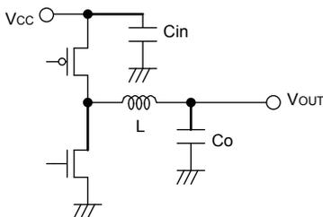
Fig.98 Input capacitor
