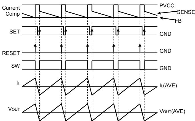
Fig.86 PWM switching timing chart
