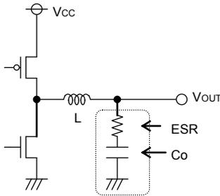
Fig.97 Output capacitor
