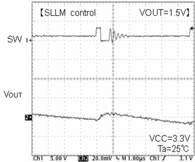
Fig.81 SW waveform I<sub>o</sub>=10mA
