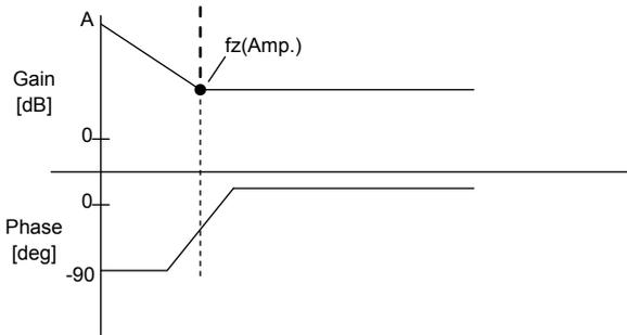
Fig.100 Error amp phase compensation characteristics
