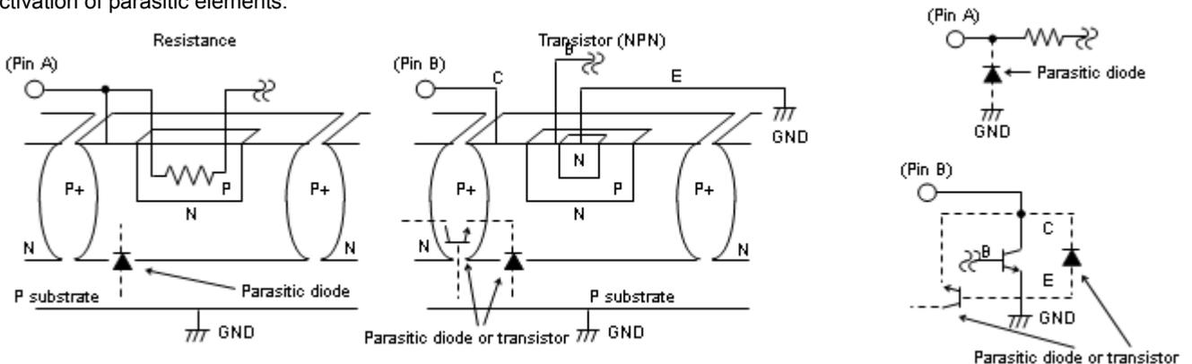
Fig.106 Simplified structure of monoristic IC
