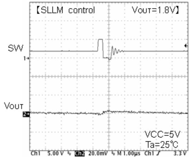
Fig.21 SW waveform  $I_o=10mA$
