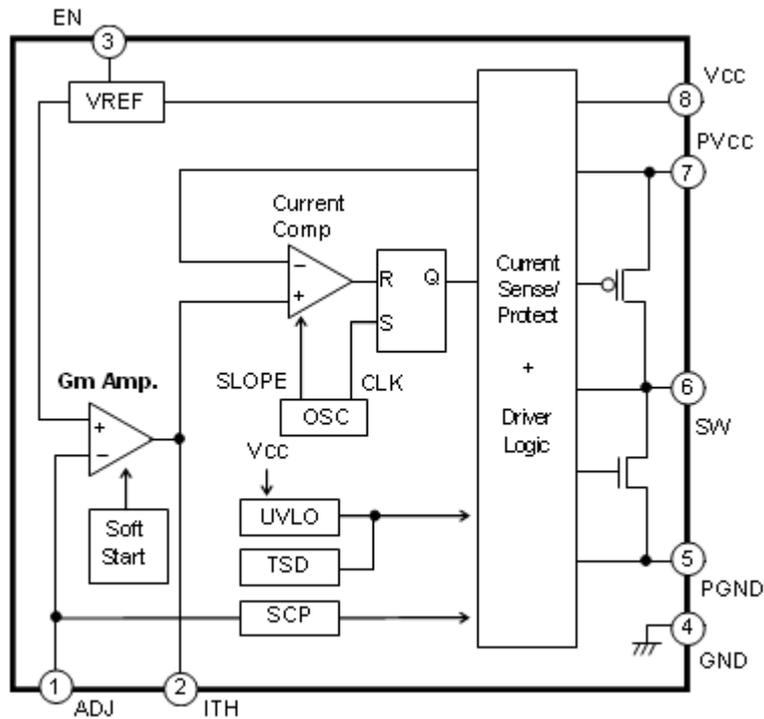
Fig.9 BD9120HFN Block Diagram
