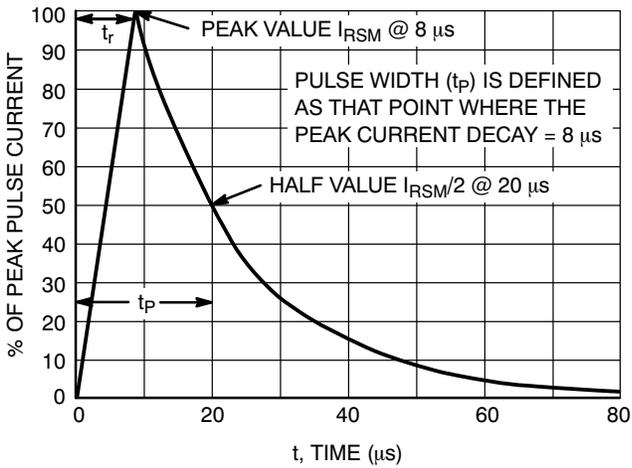
**Figure 3. 8 × 20 µs Pulse Waveform**
