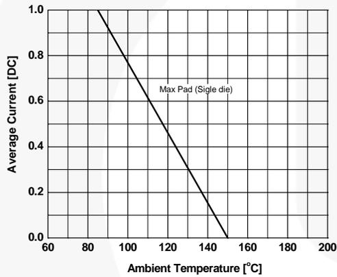
Figure 5. Maximum Average Current vs. Ambient Temperature
