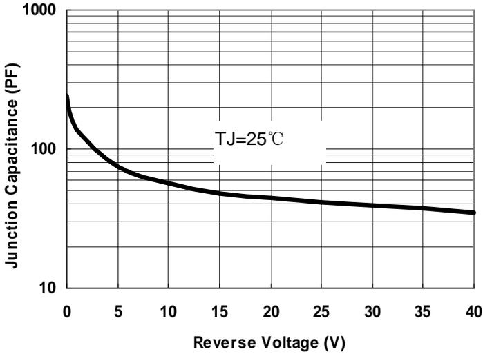
Fig.1-Typical Junction Capacitance
