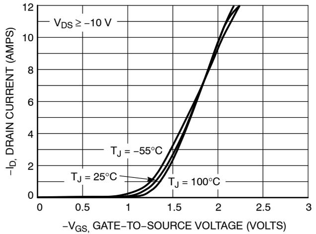
Figure 2. Transfer Characteristics
