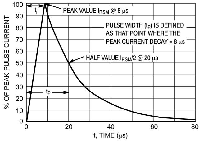
Figure 9. IEC 61000-4-5 8/20 μs Pulse Waveform
