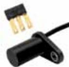
**Magnetic sensors:** Digital and analog Hall-effect position ICs, magnetoresistive position ICs, Hall-effect vane, gear-tooth, and magnetic sensors. **May be used in:** Speed and RPM sensing, motor/fan control, magnetic encoding, disc speed, tape, flow-rate sensing, conveyors, ignitions, motion control/detection, power/position, magnetic code reading, vibration, and weight sensing.
