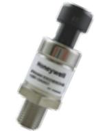
**Pressure transducers – heavy duty:** Provide a complete amplified and compensated pressure measurement solution. Choice of ports, connectors, outputs and pressure ranges, engineered to be resistant to a wide variety of media for use in most harsh environments. **May be used in:** Industrial HVAC/R and air compressors; general system and factory automation pump, valve and fluid pressure; and transportation (heavy equipment and alternative fuel vehicles) system, pneumatics, and hydraulics.
