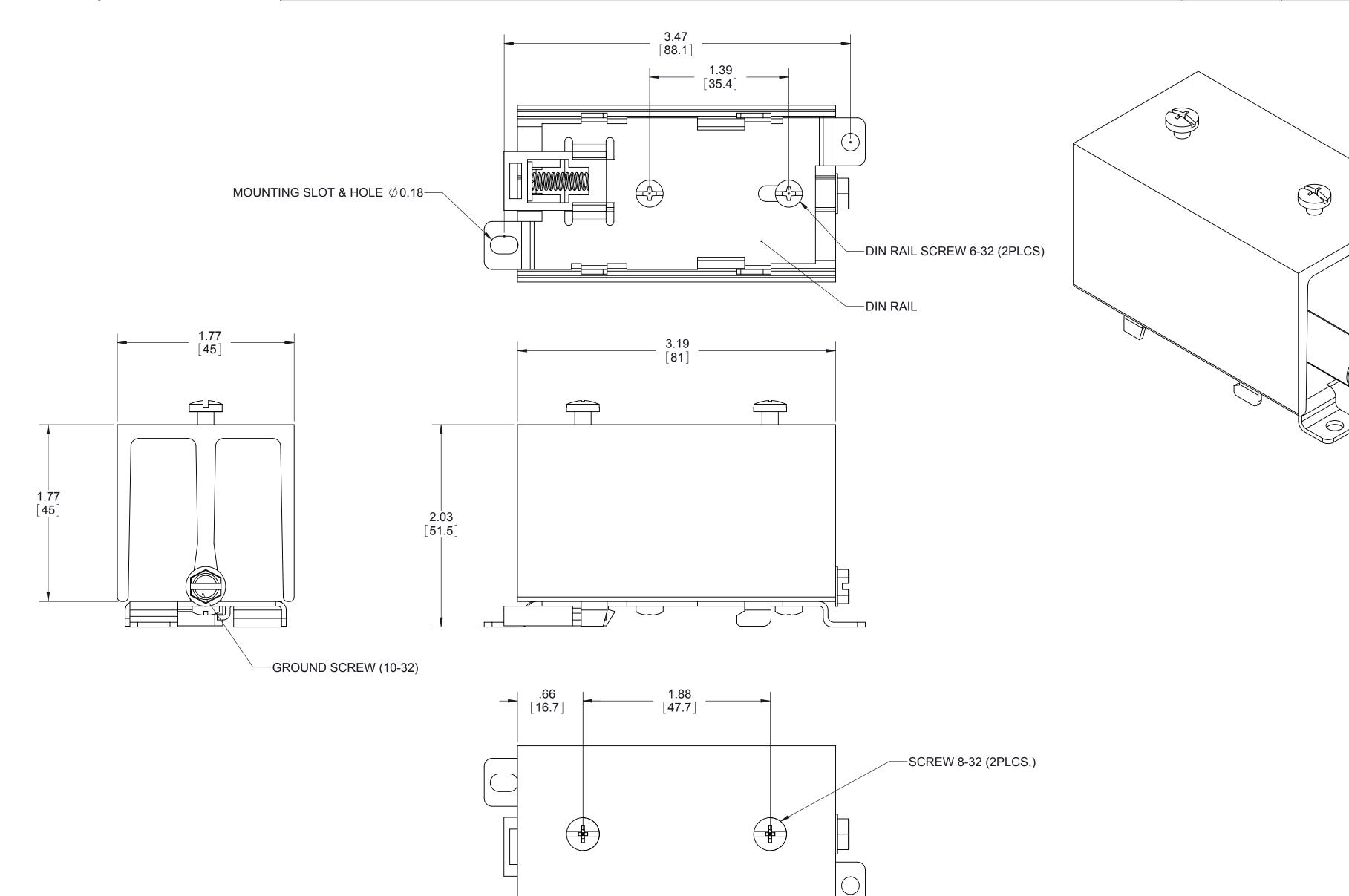
Tolerances: ± 0.02 in / 0.5 mm. All dimensions are in: inches [millimeters]
