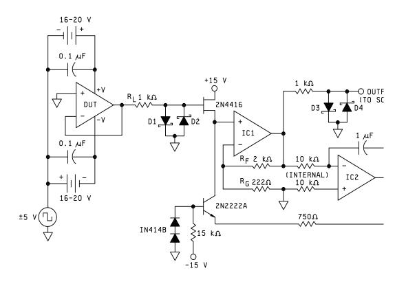
NOTES: Schottky diodes D1 – D4 are HP5082-2835 or equivalent. IC1 is CLC200A1 or equivalent. IC2 is OP41EJ or equivalent.
