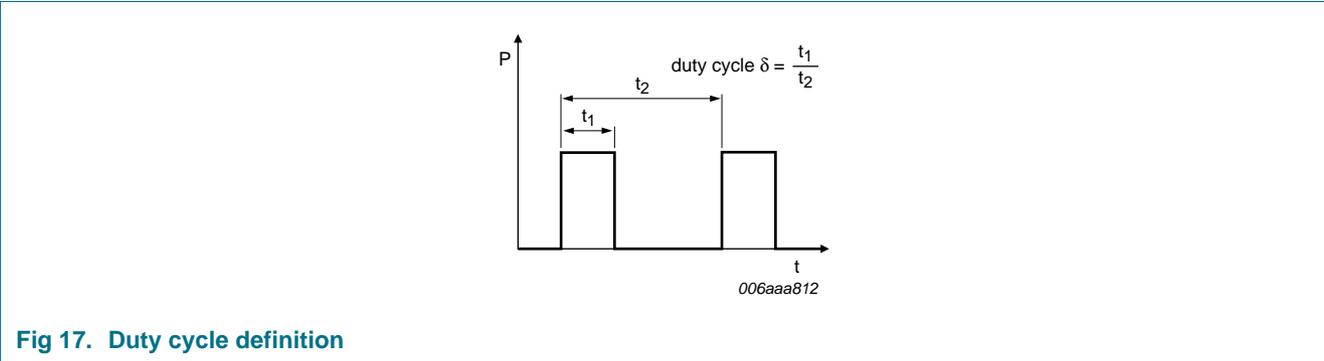
Fig 17. Duty cycle definition
