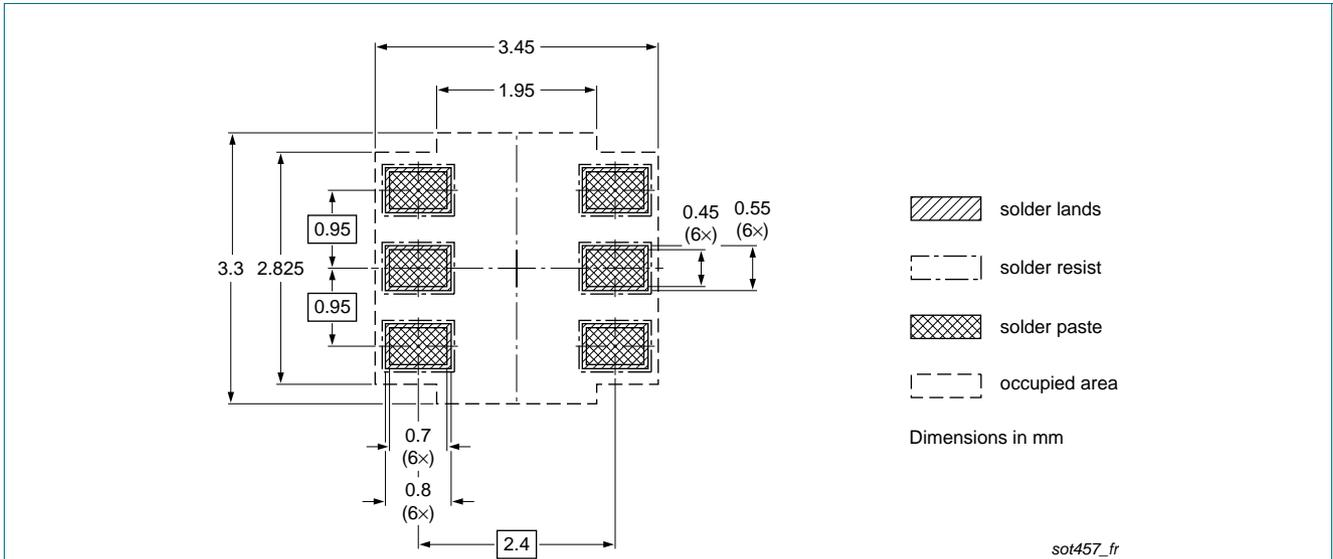
Fig 19. Reflow soldering footprint for SOT457 (TSOP6)
