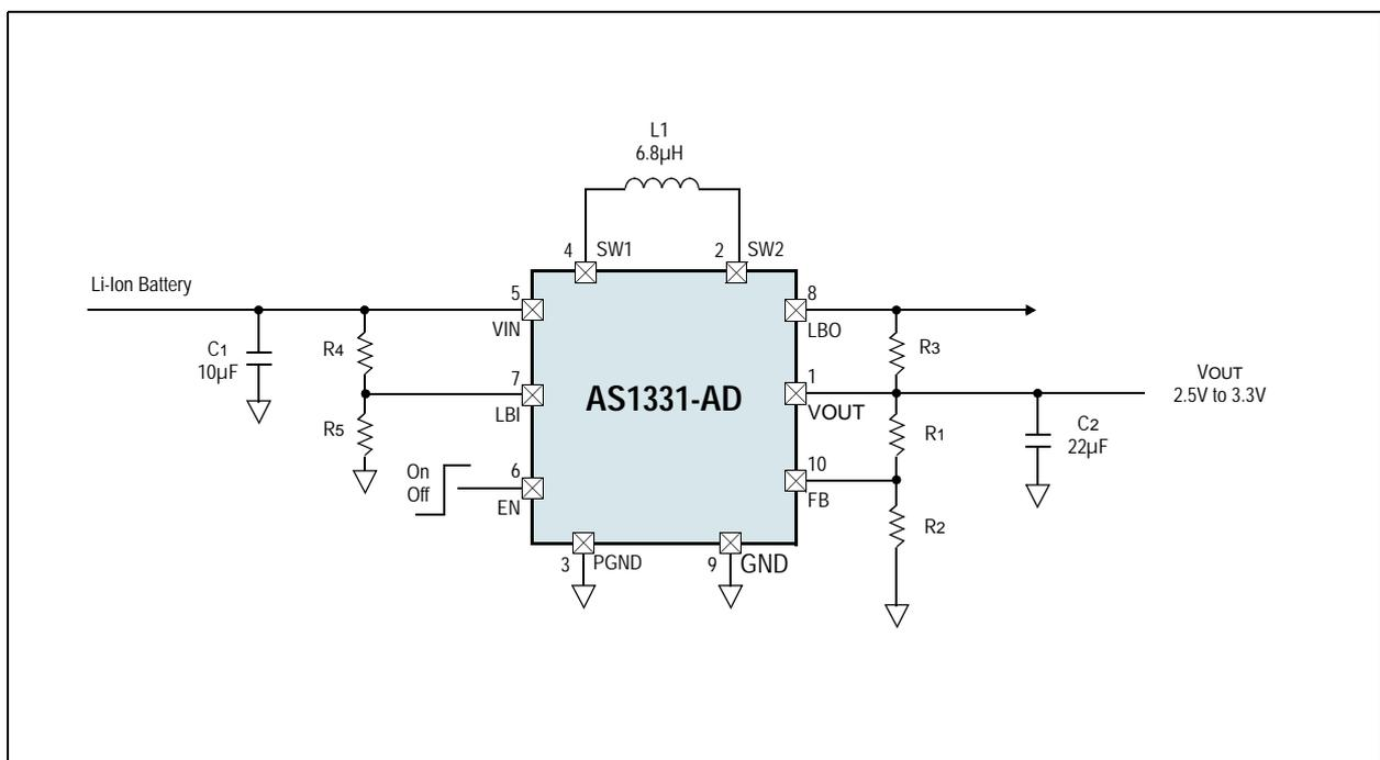
The output voltage can be adjusted by selecting different values for R1 and R2.
