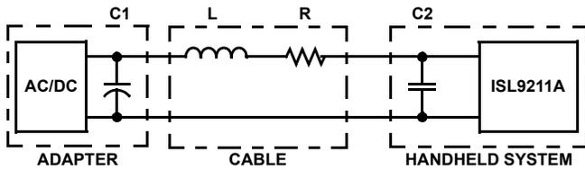
FIGURE 16. EQUIVALENT CIRCUIT FOR THE ISL9211A INPUT
