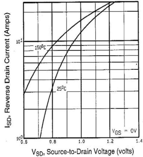
Fig. 7 - Typical Source-Drain Diode Forward Voltage
