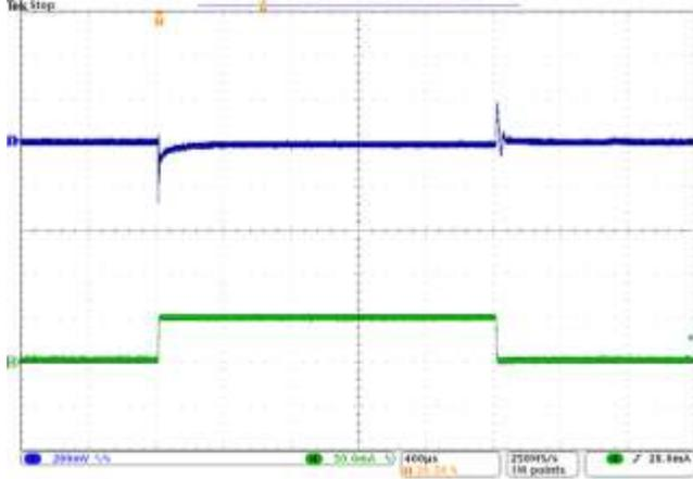
$V_{IN} = 4.3V$ ,  $V_{OUT} = 3.3V$ ,  $I_{OUT} = 50\sim 100mA$
