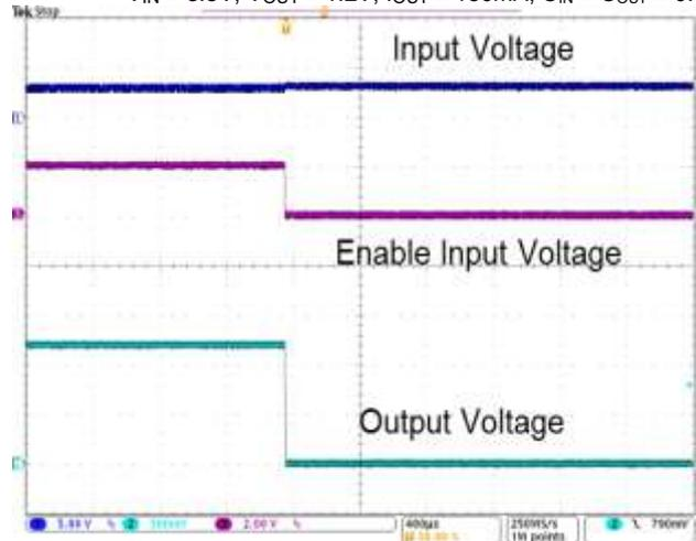
$V_{IN} = 4.3V$ ,  $V_{OUT} = 3.3V$ ,  $I_{OUT} = 0mA$ ,  $C_{IN} = C_{OUT} = 0.1\mu F$
