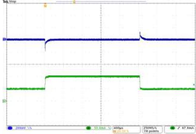
$V_{IN} = 4.3V$ ,  $V_{OUT} = 3.3V$ ,  $I_{OUT} = 1\sim 50mA$
