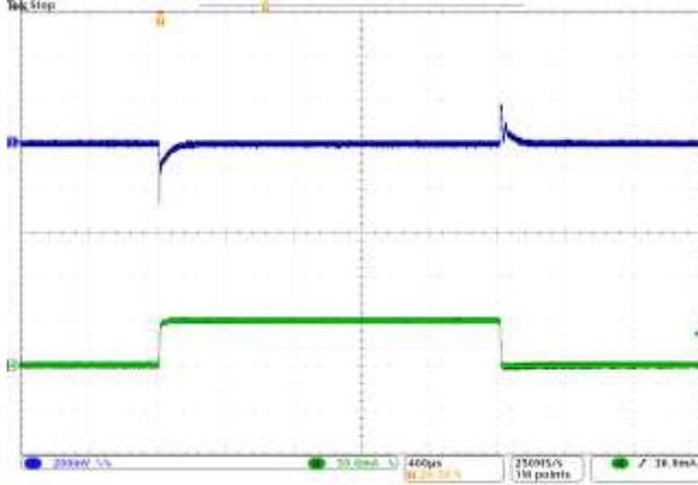
$V_{IN} = 3.3V$ ,  $V_{OUT} = 1.2V$ ,  $I_{OUT} = 50\sim 100mA$
