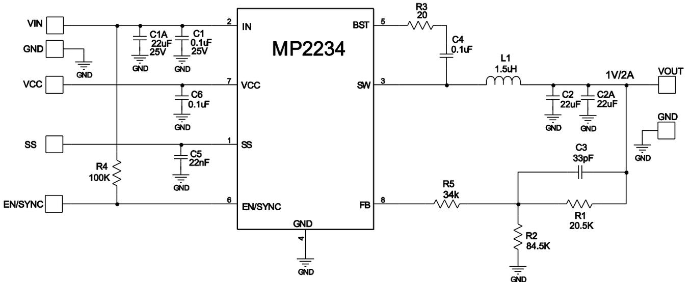
**Figure 14: 12V<sub>IN</sub>, 1V/2A Output**
