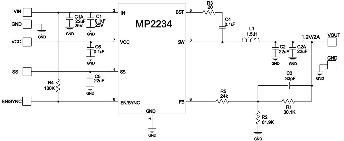
**Figure 13: 12V<sub>IN</sub>, 1.2V/2A Output**
