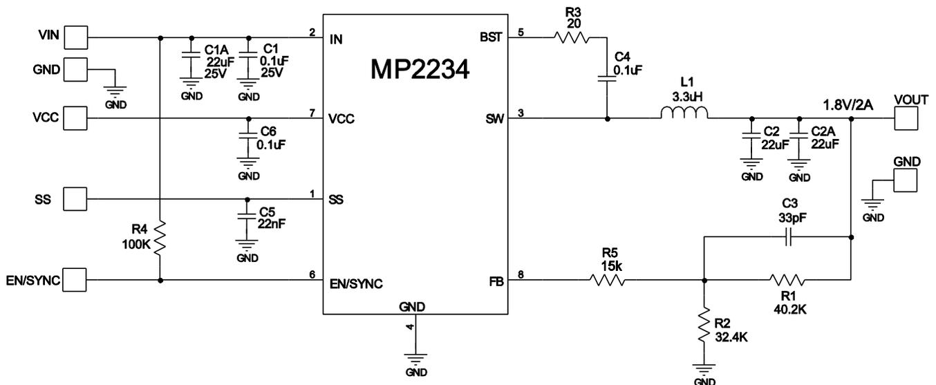
**Figure 12: 12V<sub>IN</sub>, 1.8V/2A Output**
