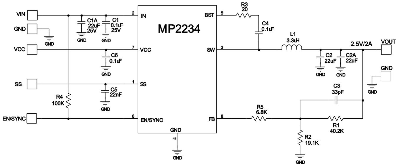
**Figure 11: 12V<sub>IN</sub>, 2.5V/2A Output**
