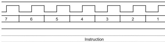
**Figure 8.26** Read Electronic Signature (RES ABh) Command Sequence
