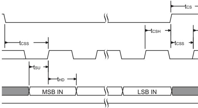
Figure 4.9 SPI Single Bit Output Timing
