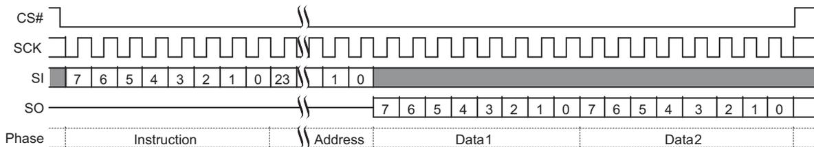
**Figure 3.6** Single Bit Wide I/O Command with Latency
