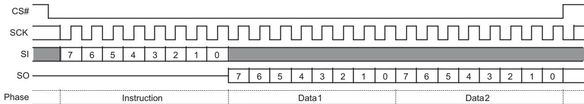
**Figure 3.5** Single Bit Wide I/O Command without Latency
