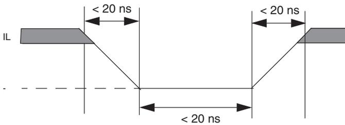
Figure 4.2 Maximum Positive Overshoot Waveform
