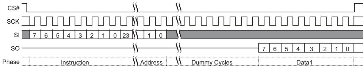
**Figure 3.7** Dual Output Command
