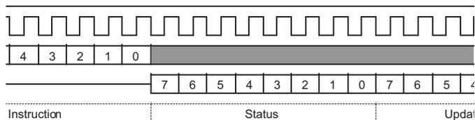
**Figure 8.2** Read Status Register-3 Command Sequence
