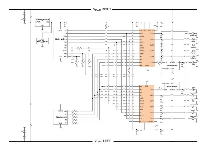
Figure 36. Typical Front Lighting Application for Automotive
