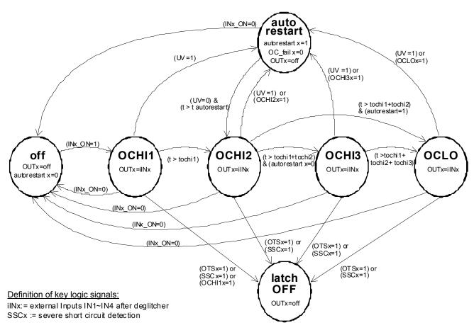
Figure 14. Output Control Diagram in Fail Mode
