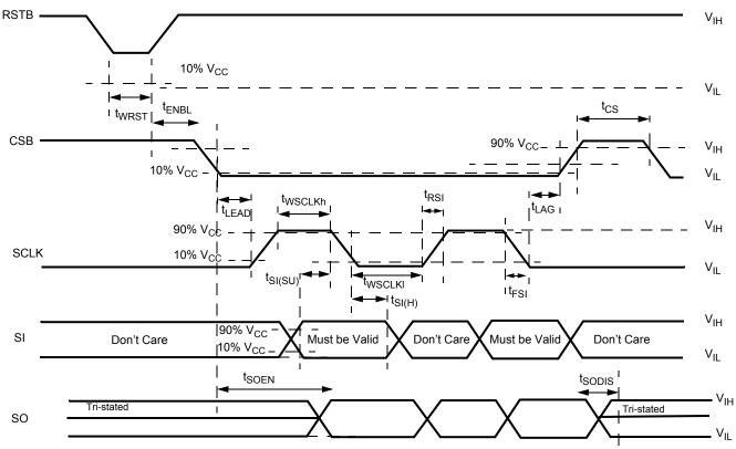
Figure 8. Timing Requirements During SPI Communication
