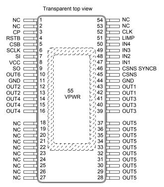
Figure 3. Pinout Diagram
