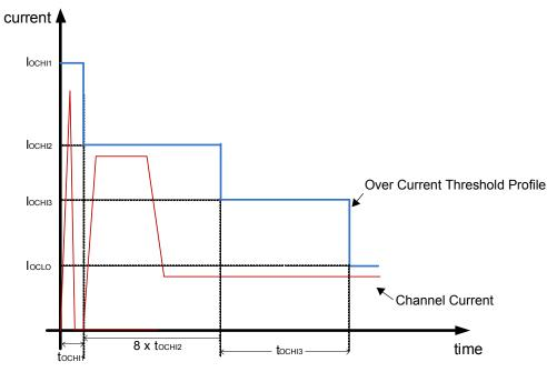
Figure 19. HID Ballast Overcurrent Profile
