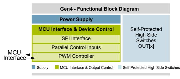
Figure 6. Functional Block Diagram
