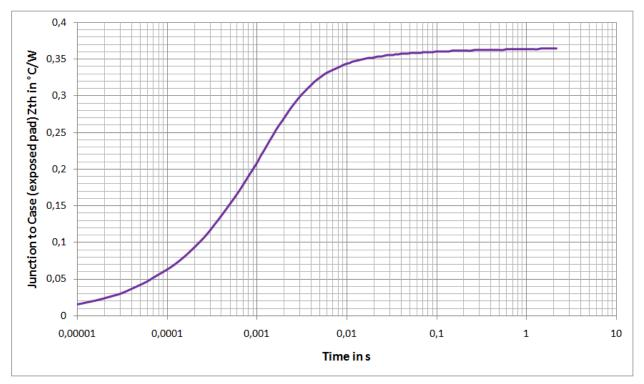
Figure 38. Transient Thermal Response Curve
