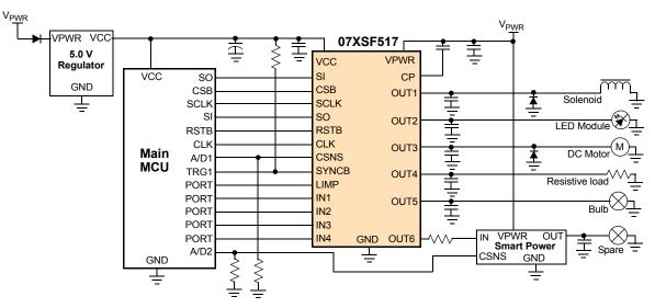
Figure 1. Triple 7.0 mOhm and Dual 17 mOhm Simplified Application Diagram
