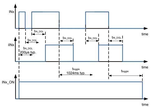
Figure 35. IN, iIN and IN\_ON signal
