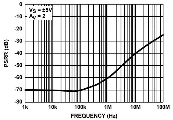
FIGURE 10. POWER SUPPLY REJECTION RATIO vs FREQUENCY
