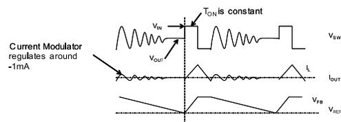
**Figure 3—Light Load Operation**
