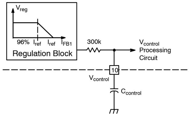
Figure 62.  $V_{control}$  Low-Pass Filtering
