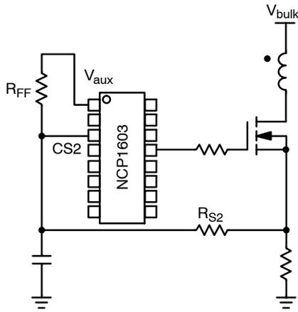
**Figure 76. Feedforward Resistor  $R_{FF}$  Added**
