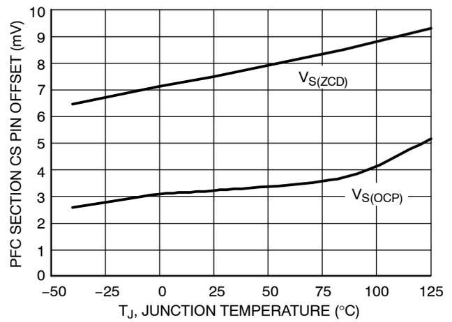
**Figure 36. PFC Section CS Pin Offset vs. Temperature**
