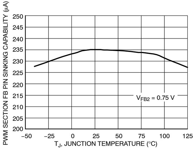
Figure 15. FB2 Pin Sinking Capability vs. Temperature
