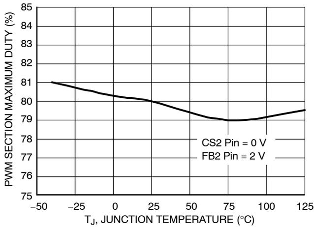
Figure 5. PWM Section Maximum Duty vs. Temperature
