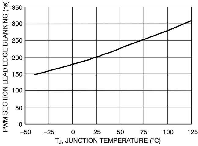
Figure 9. PWM Section Lead Edge Blanking vs. Temperature
