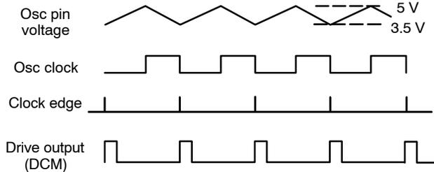
Figure 69. Oscillator Mode Timing Diagram in DCM
