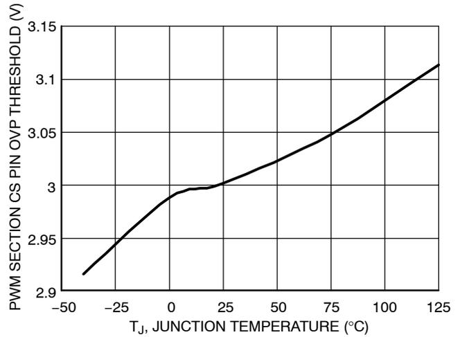
Figure 12. CS2 Pin Overvoltage Protection Threshold vs. Temperature
