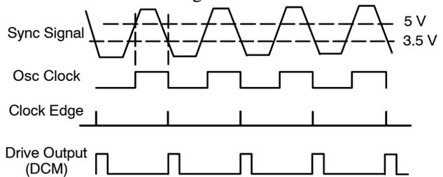
Figure 71. Synchronization Mode Timing Diagram in DCM
