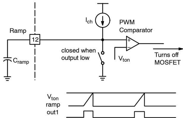
Figure 60. PFC Modulation Circuit and Timing Diagram
