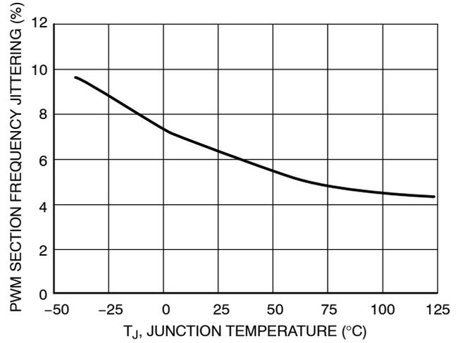
Figure 4. PWM Section Oscillator Frequency Jittering vs. Temperature
