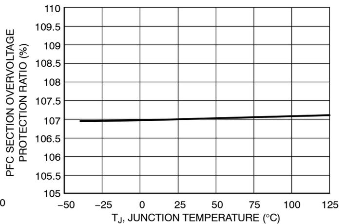
Figure 32. PFC Section Overvoltage Protection Ratio vs. Temperature
