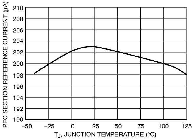
Figure 27. PFC Section Reference Current vs. Temperature
