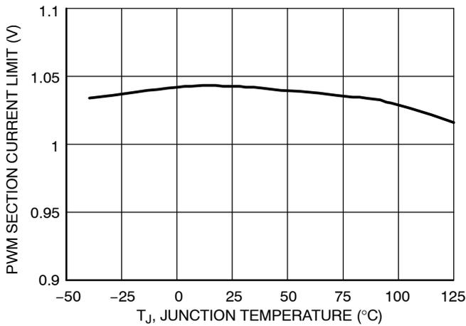
Figure 7. PWM Section Current Limit vs. Temperature
