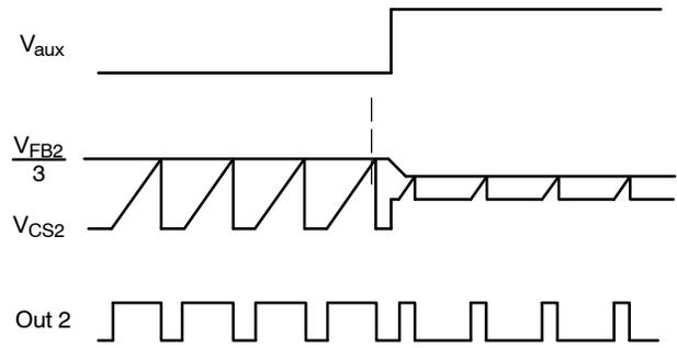
High duty when PFC is off. Low duty when PFC is on.
