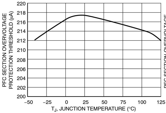
**Figure 33. PFC Section Overvoltage Protection Threshold vs. Temperature**
