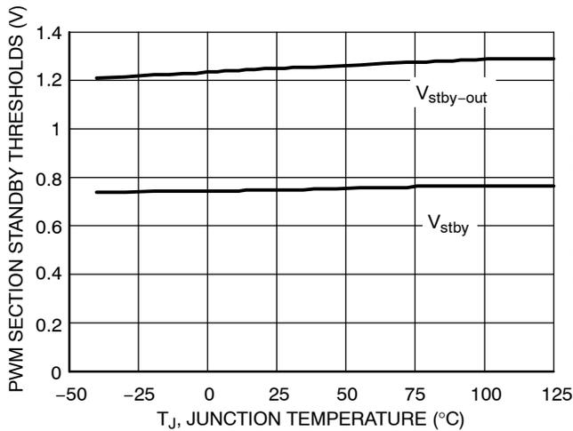
Figure 13. PWM Section Standby Thresholds vs. Temperature
