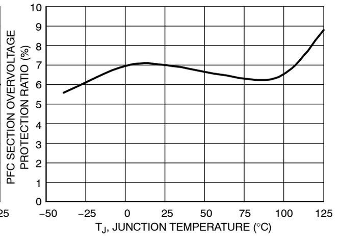
**Figure 34. PFC Section Overvoltage Protection Ratio vs. Temperature**
