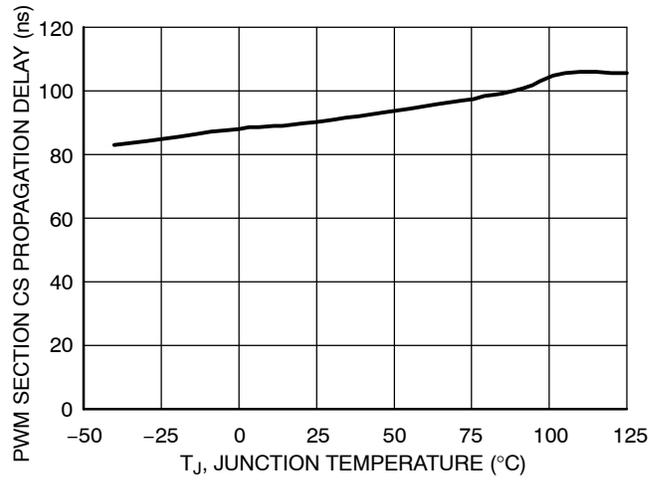
Figure 10. CS2 Pin Propagation Delay vs. Temperature
