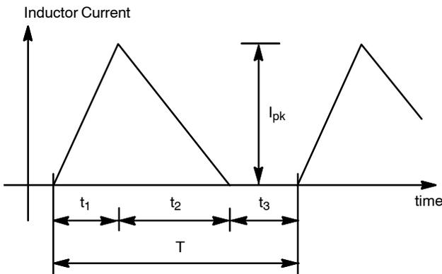
Figure 59. Inductor Current in DCM
