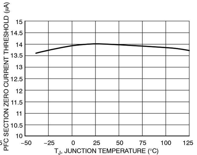
**Figure 38. PFC Section Zero Current Threshold vs. Temperature**
