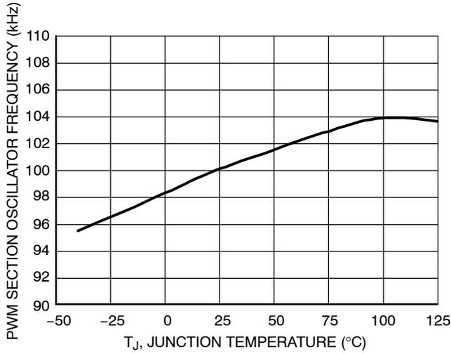
Figure 3. PWM Section Oscillator Frequency vs. Temperature
