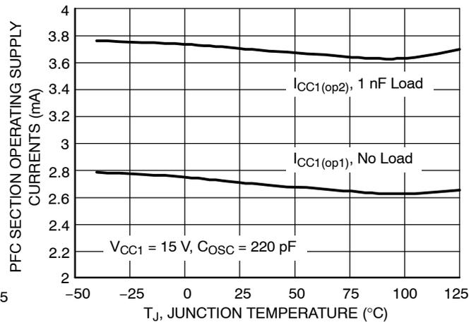
**Figure 44. PFC Section Operating Supply Currents vs. Temperature**
