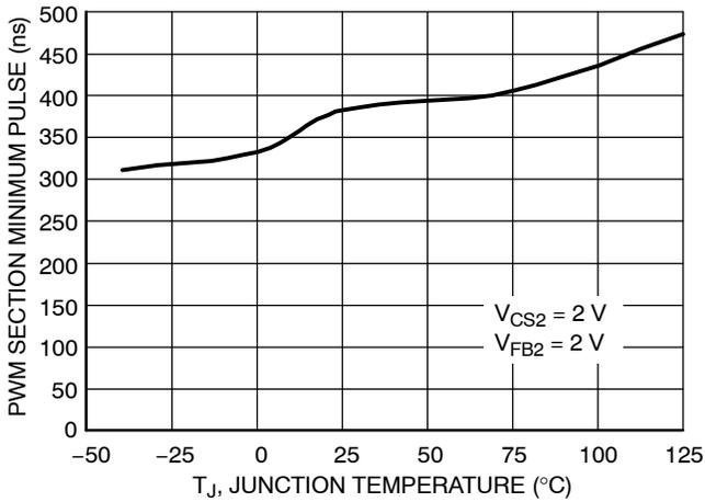
Figure 11. PWM Section Minimum Output Pulse vs. Temperature
