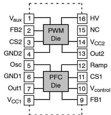
Figure 46. Internal Connection
