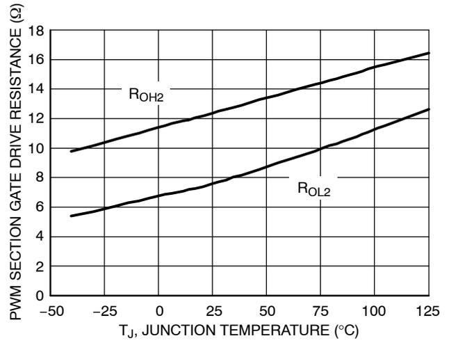
Figure 6. PWM Section Gate Drive Resistance vs. Temperature
