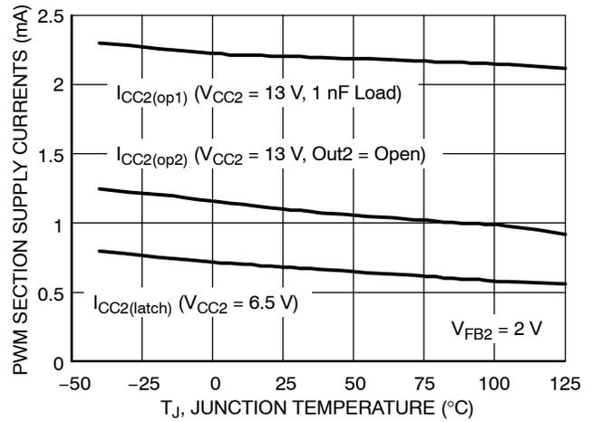
Figure 22. PWM Section Supply Currents vs. Temperature
