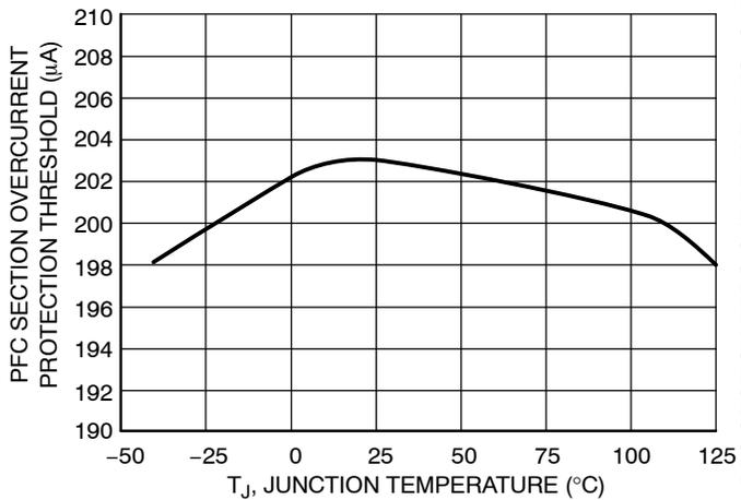
**Figure 37. PFC Section Overcurrent Protection Threshold vs. Temperature**
