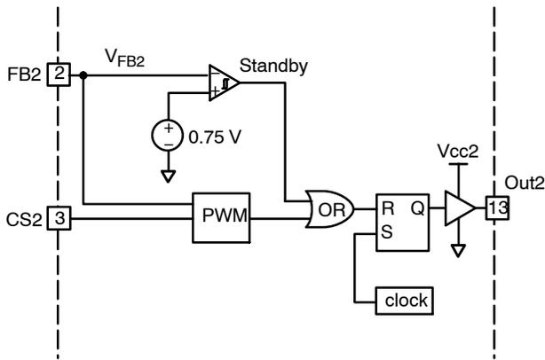
Figure 56. Block Diagram in Standby Operation in PWM Section
