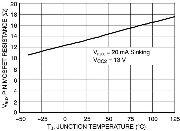
Figure 17. V<sub>aux</sub> Pin Internal MOSFET Resistance vs. Temperature
