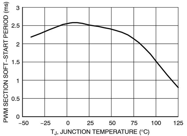
Figure 8. PWM Section Soft-Start Period vs. Temperature
