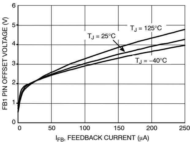
Figure 31. Feedback Pin Voltage vs. Feedback Current
