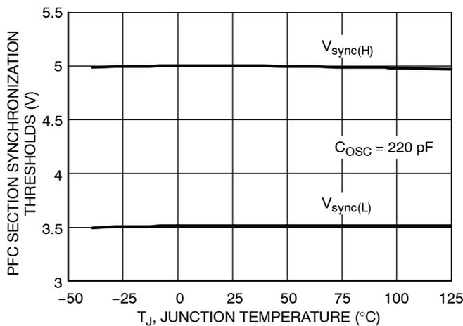
Figure 25. PFC Section Synchronization Thresholds vs. Temperature
