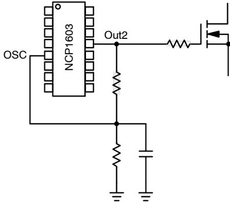
Figure 72. Synchronization Configuration
