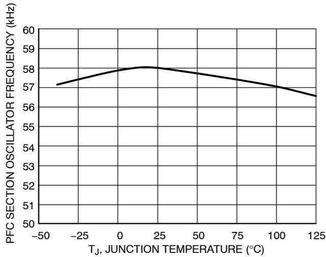
Figure 23. PFC Section Oscillator Frequency vs. Temperature
