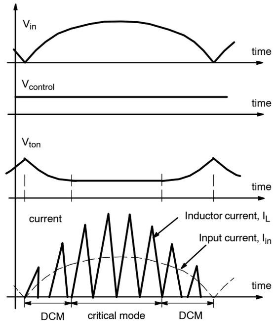
Figure 57. Timing Diagram of the PFC Stage
