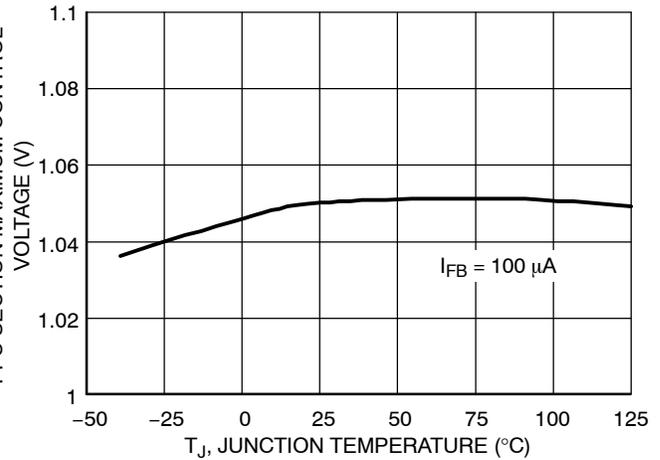
Figure 30. PFC Section Maximum Control Voltage vs. Temperature
