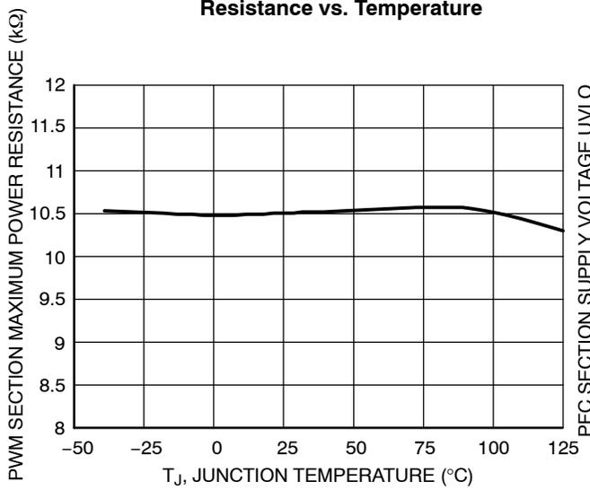
**Figure 41. PFC Section Maximum Power Resistance vs. Temperature**
