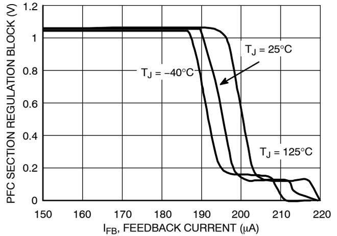
Figure 28. PFC Section Regulation Block Transfer Function
