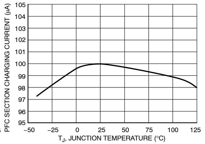
**Figure 40. PFC Section Charging Current vs. Temperature**
