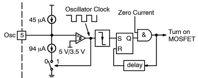
Figure 67. Oscillator / Synchronization Block in PFC Section
