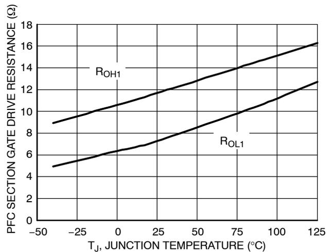
Figure 26. PFC Section Gate Drive Resistance vs. Temperature
