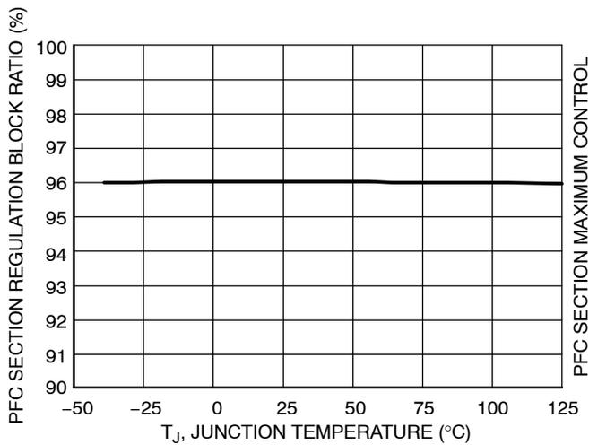
Figure 29. PFC Section Regulation Block vs. Temperature
