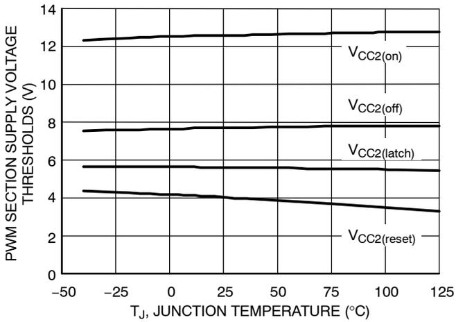
Figure 21. PWM Section Supply Voltage Thresholds vs. Temperature
