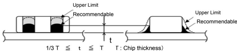
Accordingly increasing the solder volume, the mechanical stress to product is also increased.
