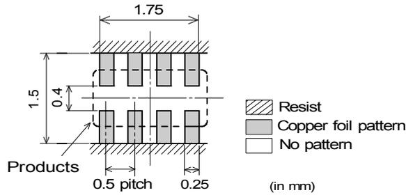
**16.7 Standard Soldering Condition (Reflow soldering)**
