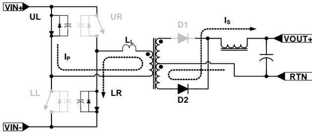
FIGURE 10. UL - LR POWER TRANSFER CYCLE
