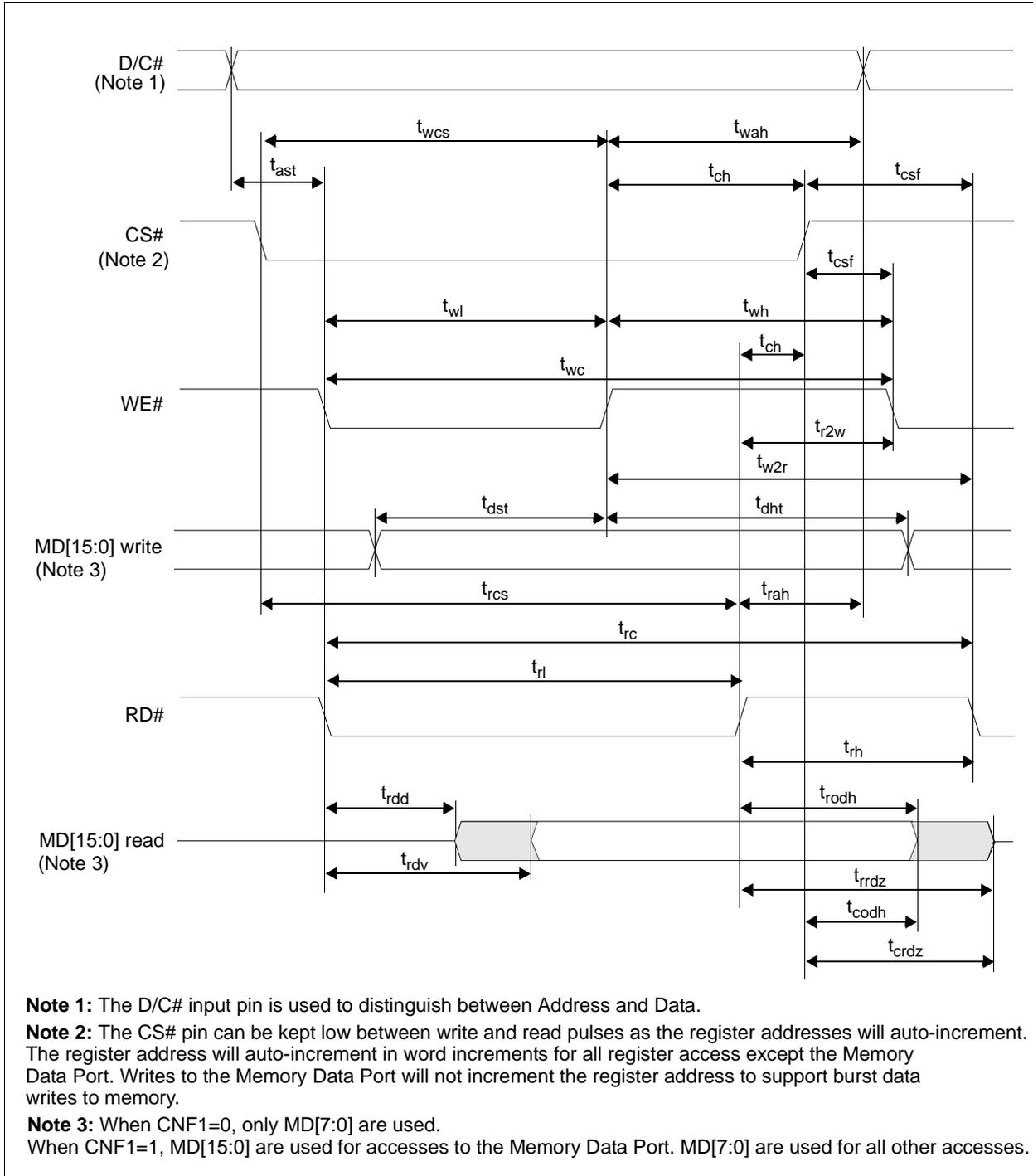
Figure 7-4: Intel 80 Input A.C. Characteristics - 1.8 Volt
