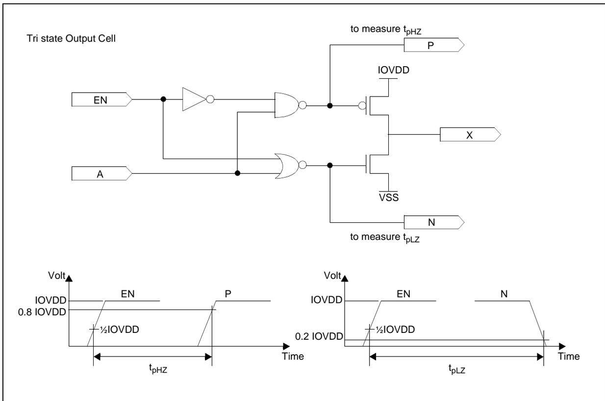
Figure 7-6: Definition of Transition Time to Hi-Z State
