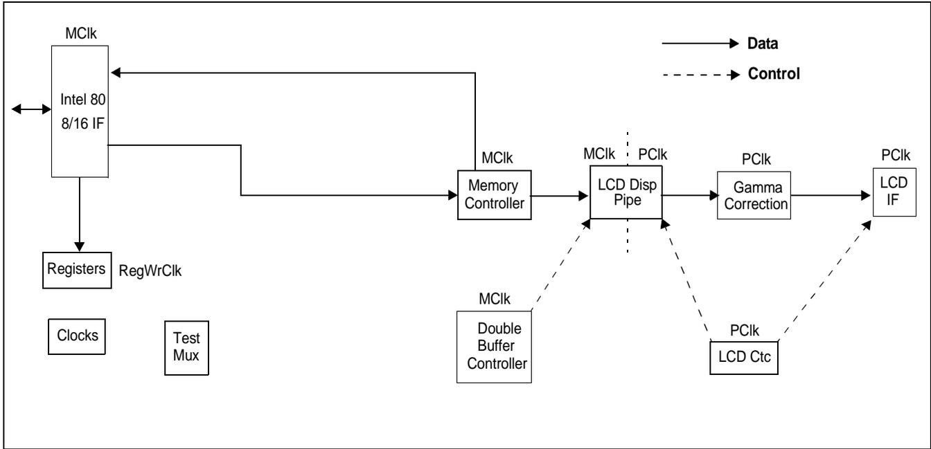
Figure 3-1: Block Diagram
