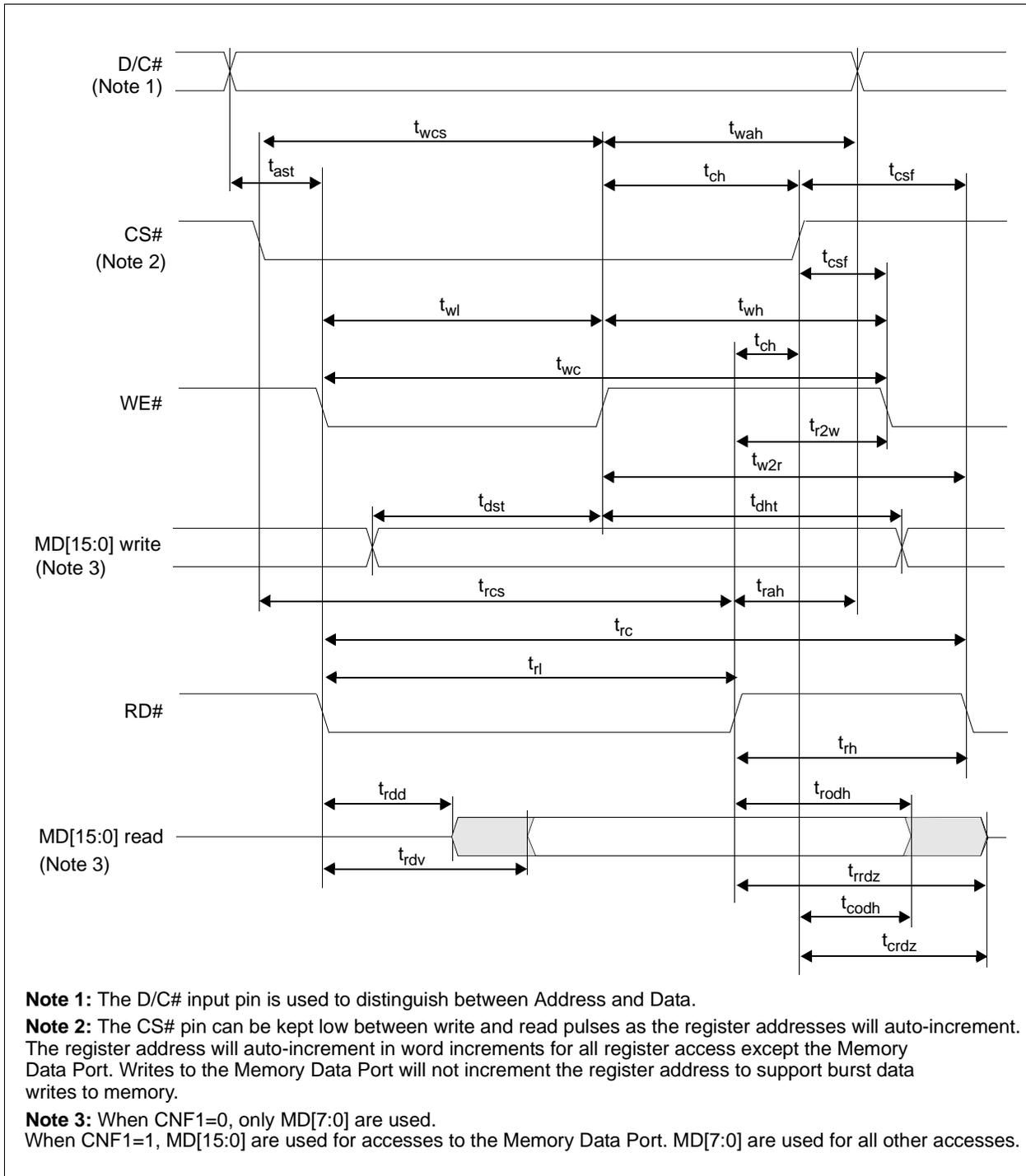
Figure 7-5: Intel 80 Input A.C. Characteristics - 3.3 Volt
