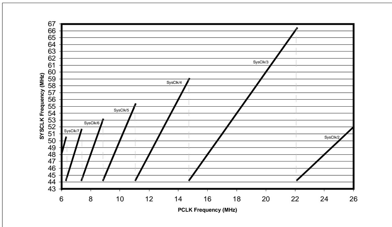
Figure 8-3: Setting of SYSCLK For a Desired PCLK
