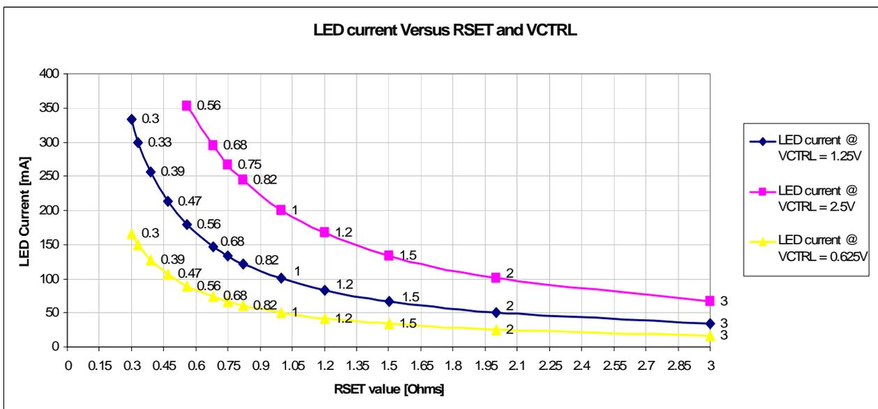
Figure 4 LED Current Setting vs. R<sub>SET</sub> and V<sub>CTRL</sub>
