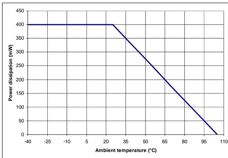
**Figure 8 Derating Curve**
