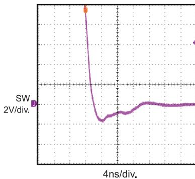
**Input/Output Voltage Ripple**
