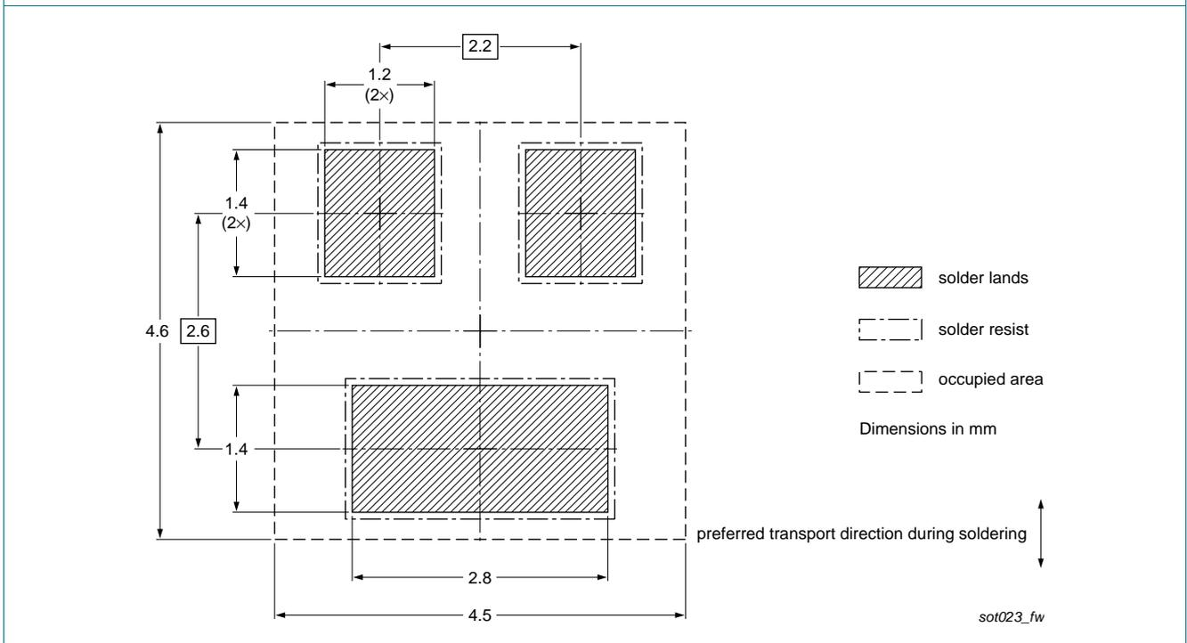
Fig 20. Wave soldering footprint for SOT23 (TO-236AB)
