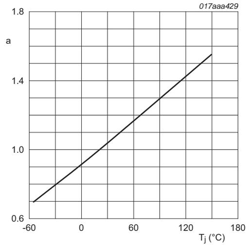
$$a = \frac{R_{DSon}}{R_{DSon(25^\circ\text{C})}}$$
