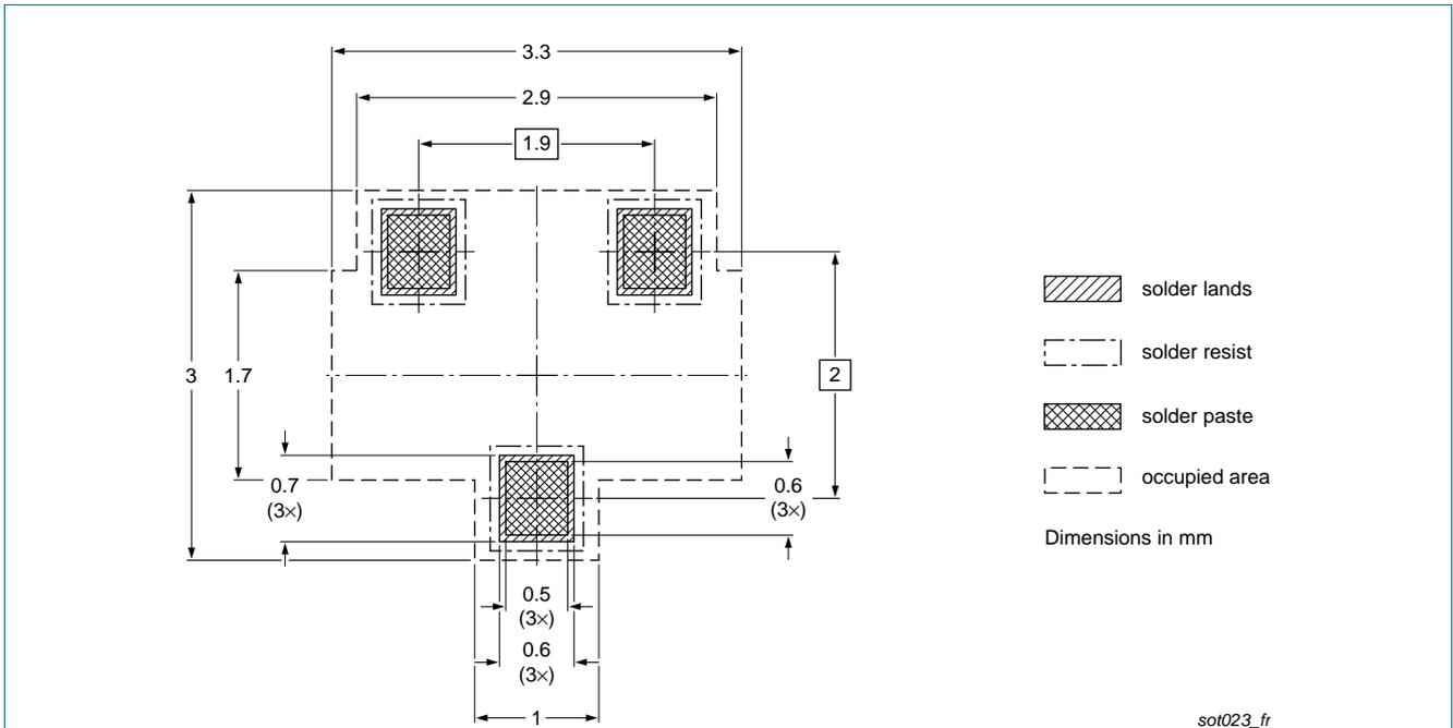
Fig 19. Reflow soldering footprint for SOT23 (TO-236AB)
