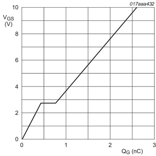
$I_D = 1.9 \text{ A}; V_{DS} = 15 \text{ V}; T_{amb} = 25 \text{ }^\circ\text{C}$
