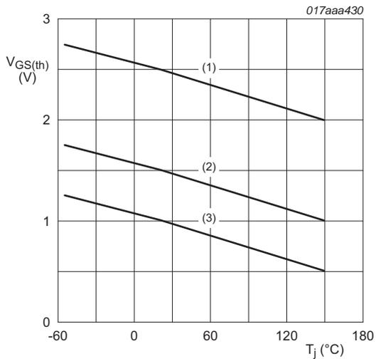
$I_D = 0.25\text{ mA}; V_{DS} = V_{GS}$
