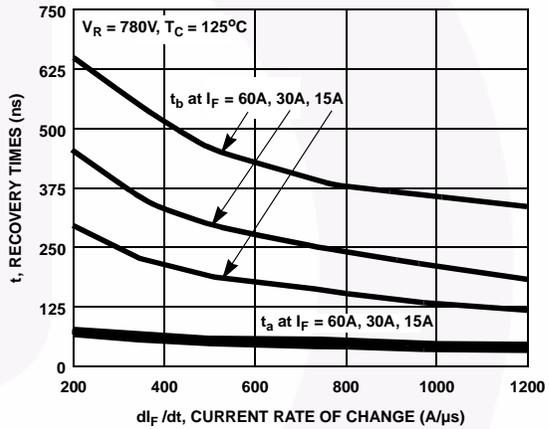
Figure 4.  $t_a$  and  $t_b$  Curves vs  $di_F/dt$
