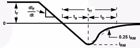
Figure 14.  $t_{tr}$  Waveforms and Definitions
