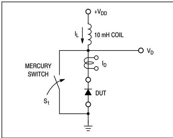
Figure 11. Test Circuit
