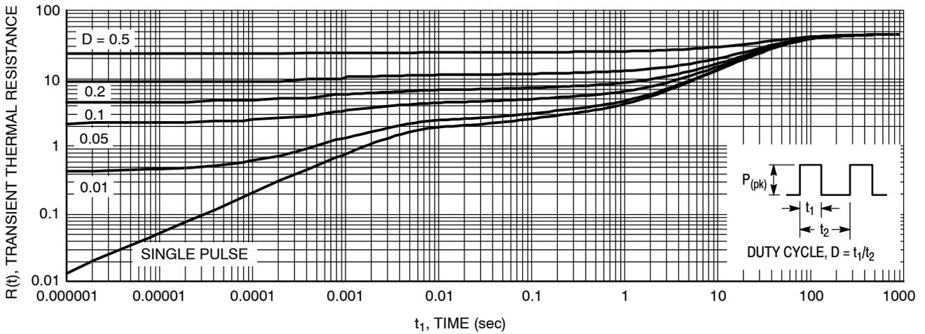
**Figure 8. Thermal Response Junction-to-Ambient for MBR20H100CT, MBRB20H100CT and NRVBB20H100CTT4G**
