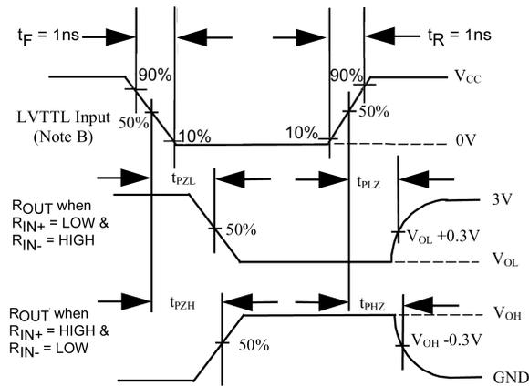
FIGURE 3. LVTTTL Outputs Test Circuit and AC Waveforms
