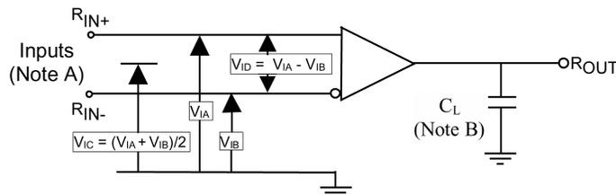
**Note A:** All differential input pulses have frequency = 10MHz,  $t_R$  or  $t_F = 1\text{ ns}$
