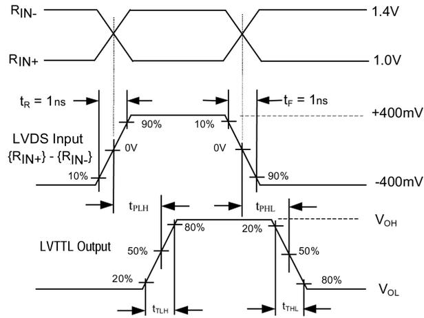
FIGURE 2. LVDS Input to LVTTTL Output AC Waveforms
