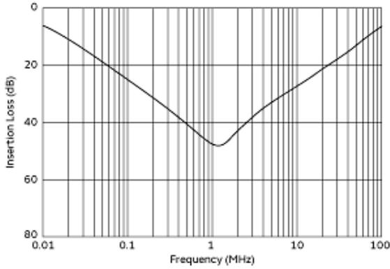
Common Mode Insertion Loss (Typ.)
