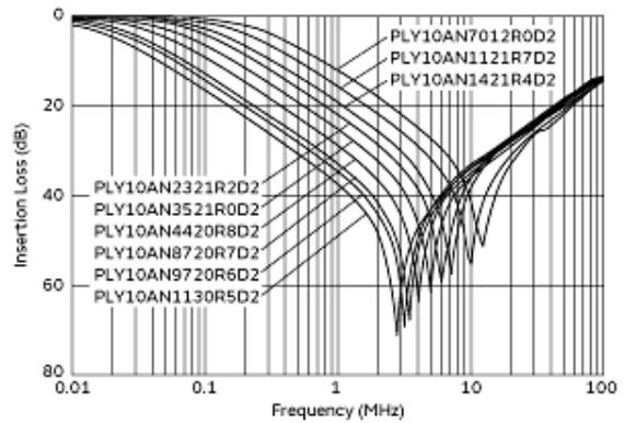
Differential Mode Insertion Loss-Frequency Characteristics
