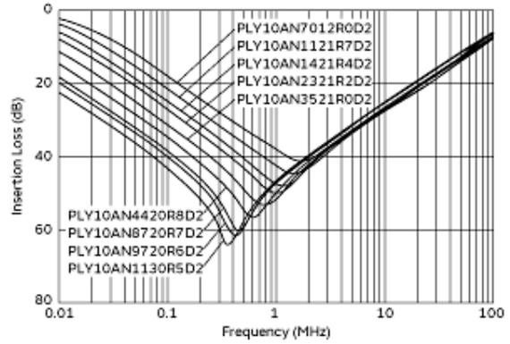
Common Mode Insertion Loss-Frequency Characteristics
