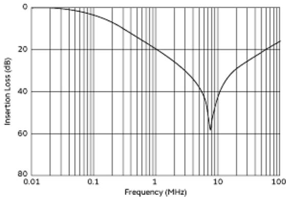
Differential Mode Insertion Loss (Typ.)
