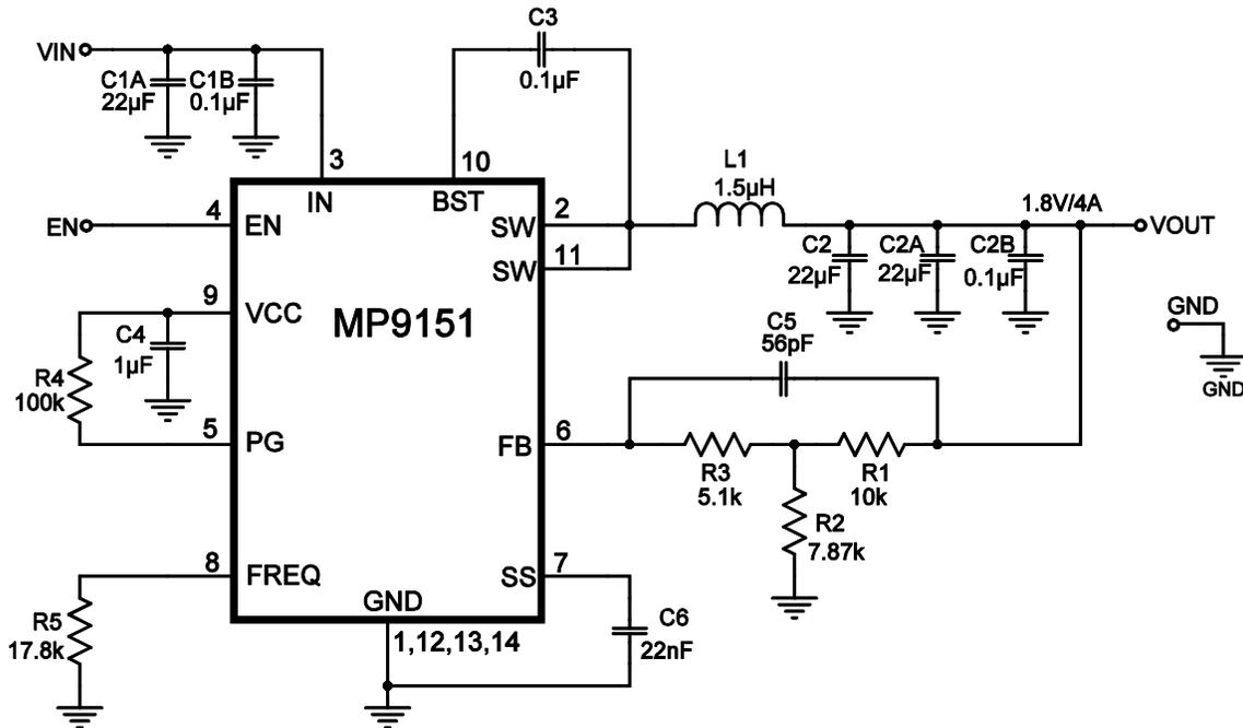
Figure 10: 800kHz, 12V<sub>IN</sub>, 1.8V/4A Output
