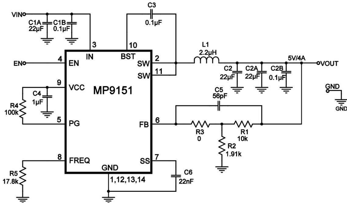
Figure 7: 800kHz, 12V<sub>IN</sub>, 5V/4A Output
