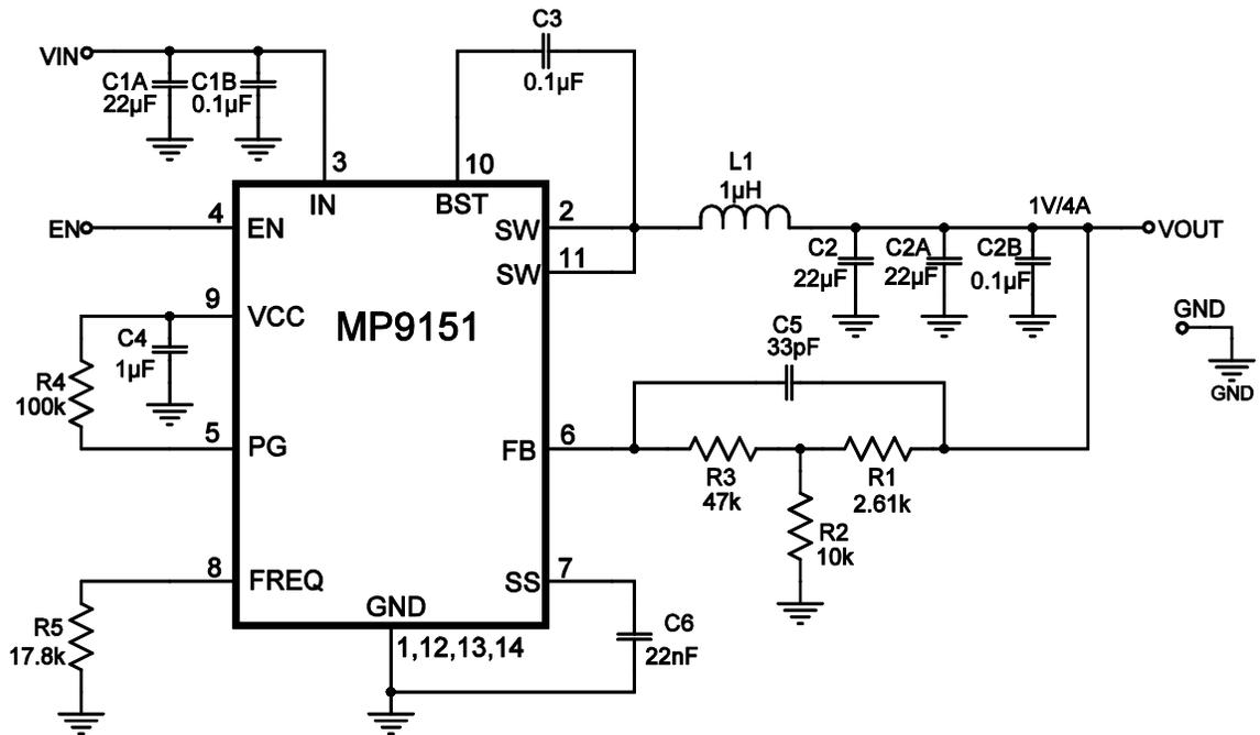
**Figure 12: 800kHz, 12V<sub>IN</sub>, 1V/4A Output**
