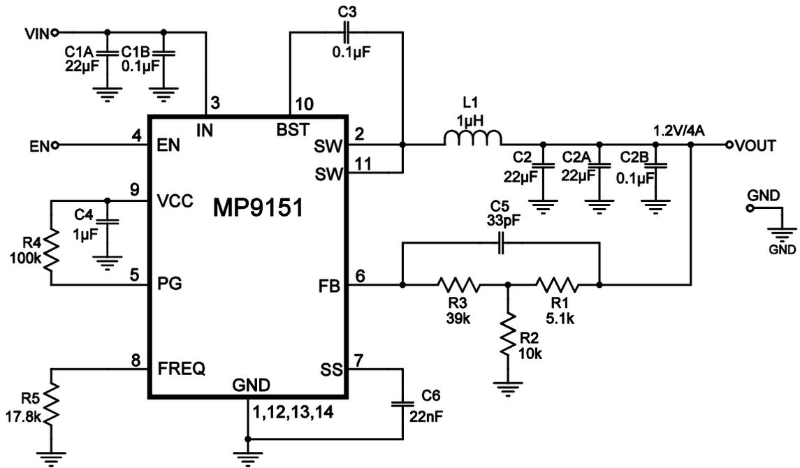
**Figure 11: 800kHz, 12V<sub>IN</sub>, 1.2V/4A Output**
