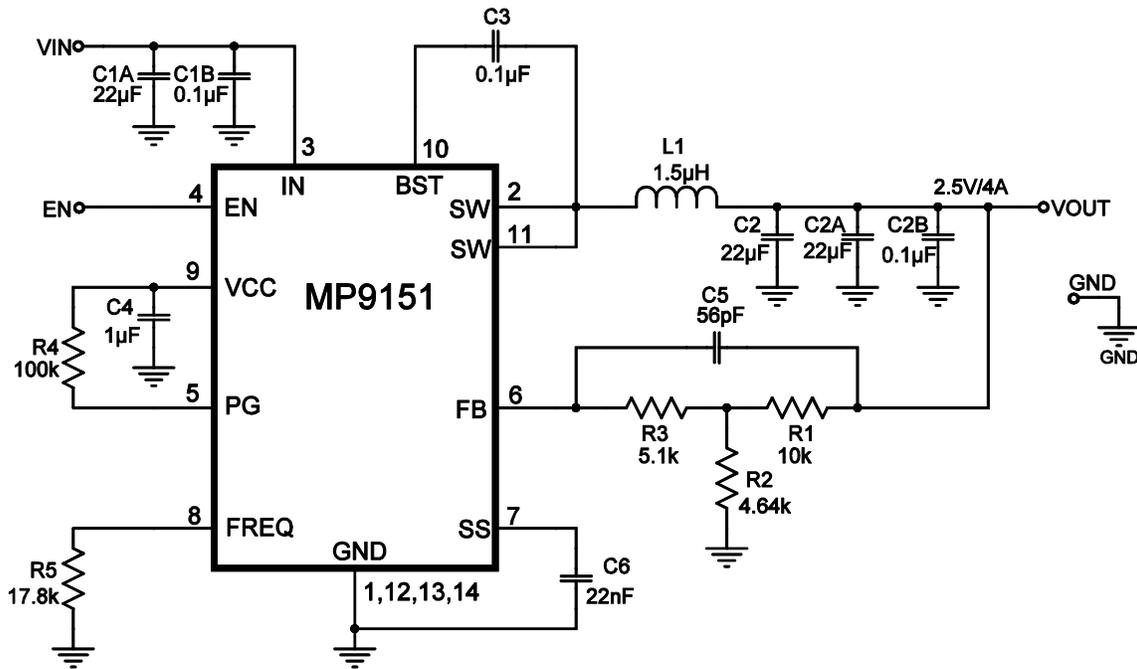
Figure 9: 800kHz, 12V<sub>IN</sub>, 2.5V/4A Output
