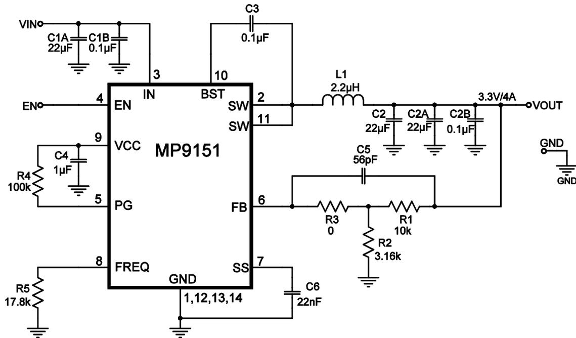
Figure 8: 800kHz, 12V<sub>IN</sub>, 3.3V/4A Output
