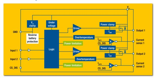
According to the innovative protection strategy introduced in VIPower™ M0-5 technology, the VND5004B is equipped with power limitation control removing the thermal fatigue, main cause of silicon degradation. Moreover, under reverse battery condition the device is protected by PowerMOS reactivation.
