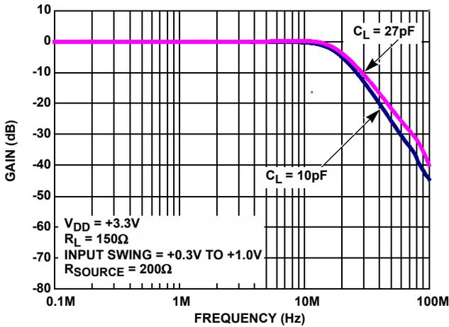
FIGURE 3. GAIN vs FREQUENCY FOR VARIOUS  $C_{LOAD}$
