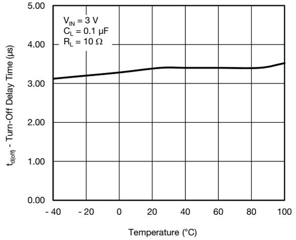
Fig. 20 - Turn-Off Delay Time vs. Temperature
