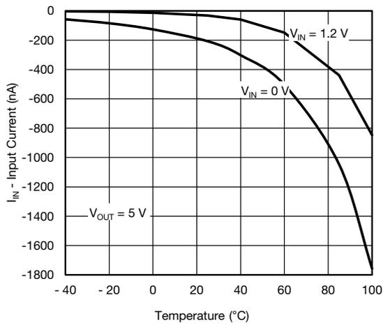
Fig. 14 - Reverse Blocking Current vs. Temperature
