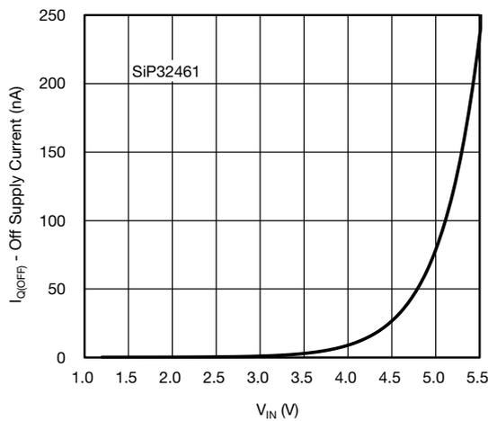
Fig. 4 - Off Supply Current vs. Input Voltage
