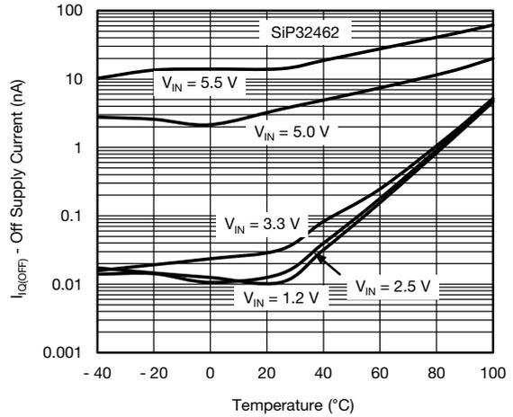
Fig. 10 - Off Supply Current vs. Temperature
