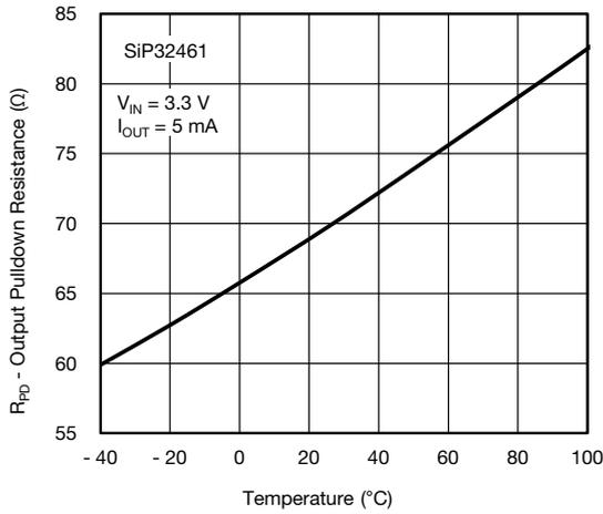
Fig. 19 - Output Pulldown Resistance vs. Temperature
