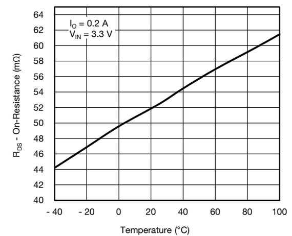
Fig. 12 -  $R_{DS(on)}$  vs. Temperature
