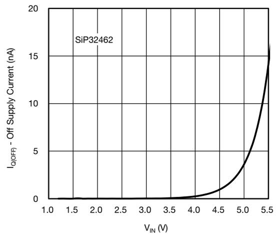
Fig. 6 - Off Supply Current vs. Input Voltage
