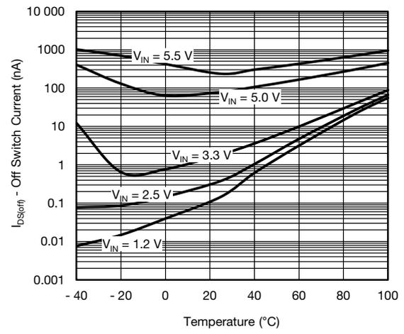
Fig. 11 - Off Switch Current vs. Temperature
