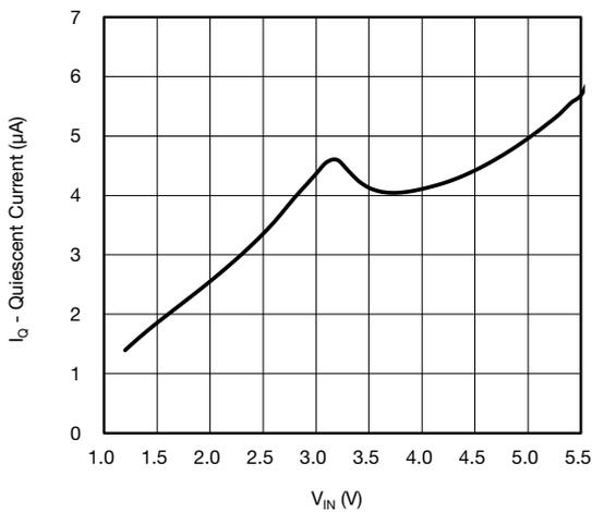
Fig. 3 - Quiescent Current vs. Input Voltage
