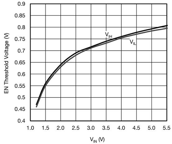
Fig. 16 - EN Threshold Voltage vs. Input Voltage
