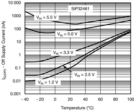
Fig. 7 - Off Supply Current vs. Temperature
