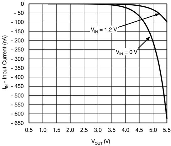
Fig. 13 - Reverse Blocking Current vs. Output Voltage
