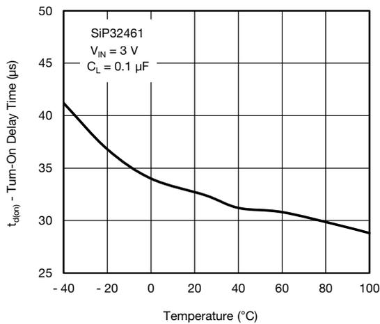
Fig. 15 - Turn-On Delay Time vs. Temperature
