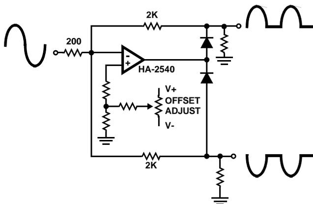
NOTE: With one HA-2540 and two low capacitance switching diodes, signals exceeding 10MHz can be separated. This circuit is most useful for full wave rectification, AM detectors or sync generation.
