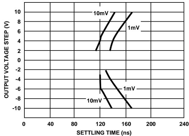
FIGURE 9. SETTLING TIME FOR VARIOUS OUTPUT STEP VOLTAGES
