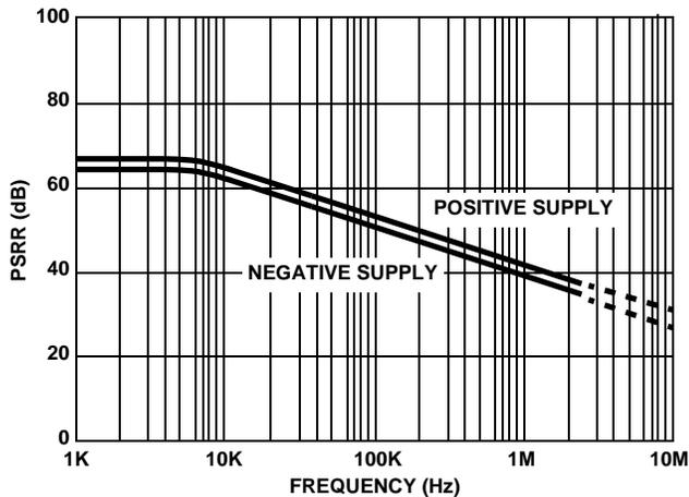
FIGURE 15. POWER SUPPLY REJECTION RATIO vs FREQUENCY
