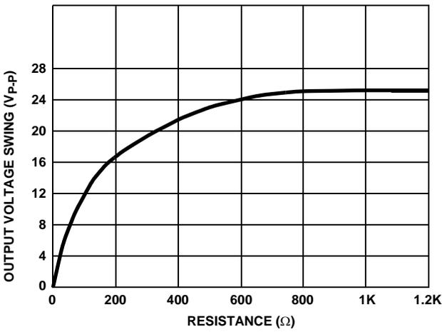
FIGURE 7. OUTPUT VOLTAGE SWING vs LOAD RESISTANCE
