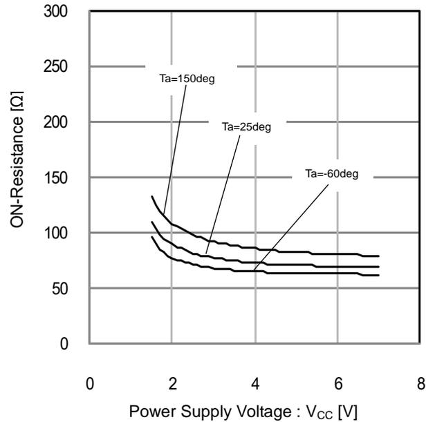
Figure 16. ON-Resistance vs Power Supply Voltage (V<sub>STB</sub>=0V) (V<sub>out</sub> discharge SW)
