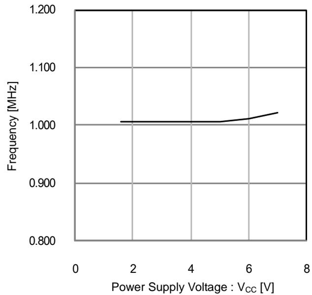
Figure 4. Oscillation Frequency vs Power Supply Voltage
