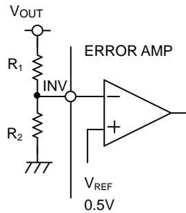
$$V_{OUT} = \frac{(R_1 + R_2)}{R_2} \times 0.5 \quad [V] \quad (6)$$
