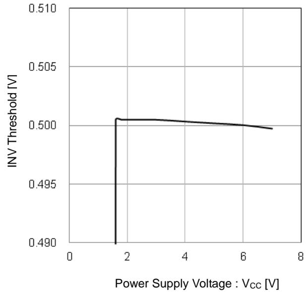
Figure 2. INV Threshold vs Power Supply Voltage
