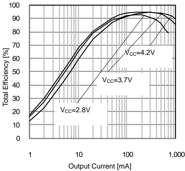
Figure 31. Total Efficiency vs Output Current
