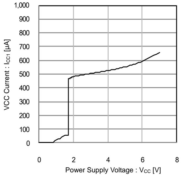
Figure 14. VCC Input Current vs Power Supply Voltage (V<sub>INV</sub>=0.8V, stop DC/DC)
