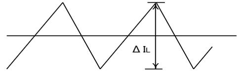
Figure 37. Ripple Current
