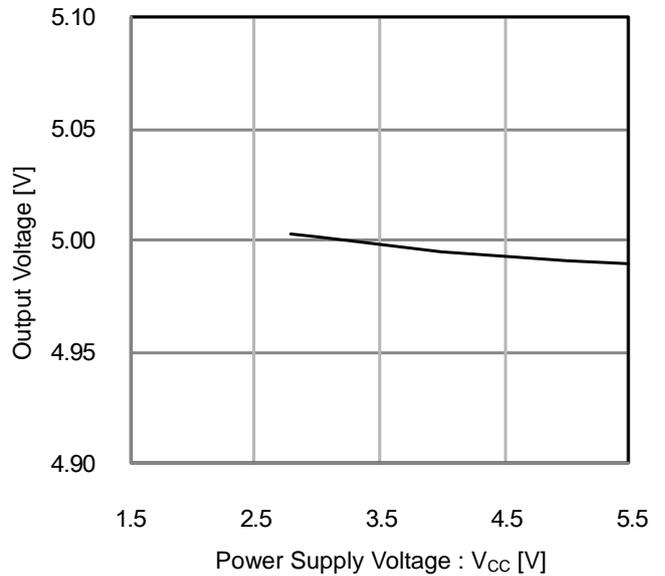
Figure 32. Output Voltage vs Power Supply Voltage
