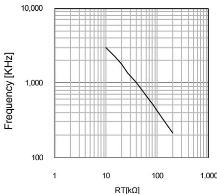
Figure 38. Oscillation Frequency vs RT Pin Resistance
