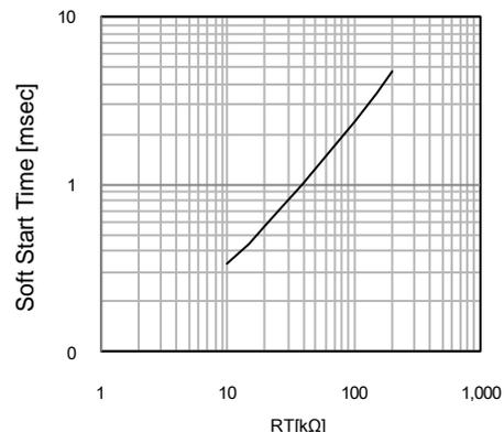
Figure 39. Soft-Start Time vs RT Pin Resistance
