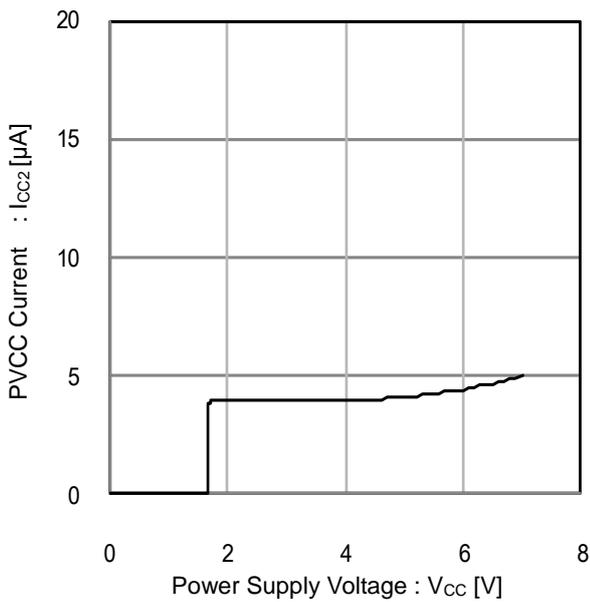
Figure 15. PVCC Input Current vs Power Supply Voltage (V<sub>INV</sub>=0.8V, stop DC/DC)
