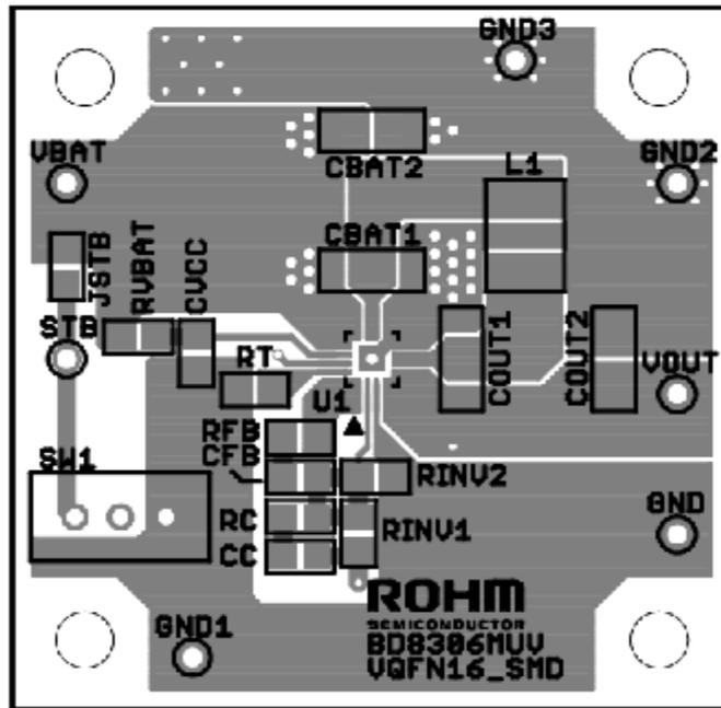
Figure 20. Assembly Layer
