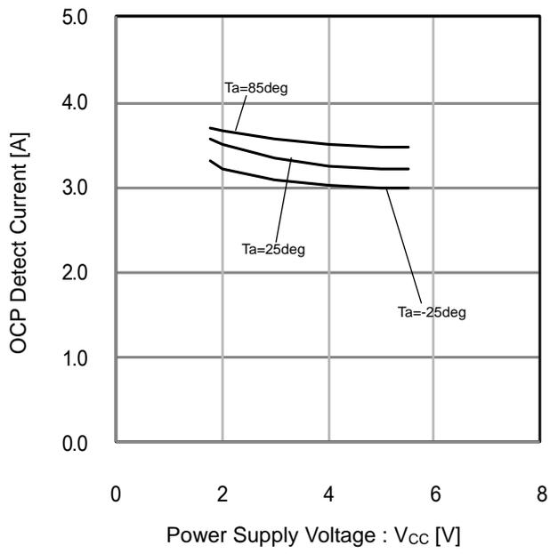
Figure 17. OCP Detect Current vs Power Supply Voltage
