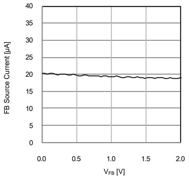
Figure 8. FB Source Current vs  $V_{FB}$  ( $V_{INV}=0.2V$ )
