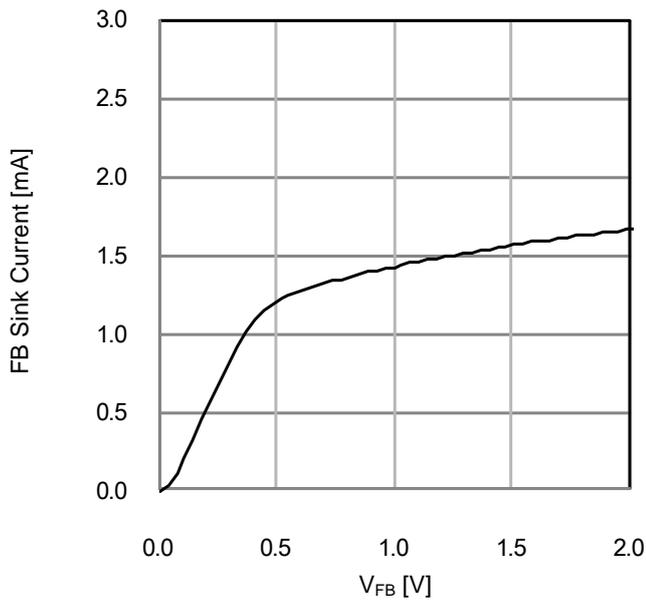
Figure 7. FB Sink Current vs  $V_{FB}$  ( $V_{INV}=0.8V$ )
