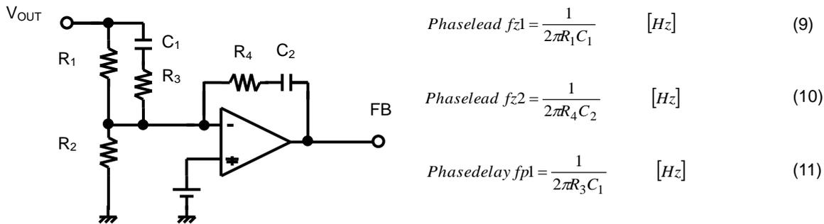
Figure 43. Example of Setting of Phase Compensation
