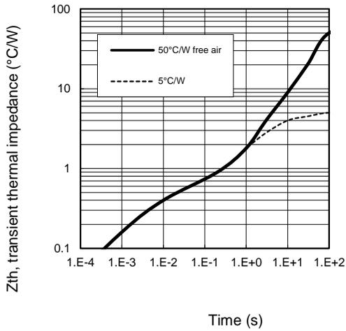
**Figure 14 – Transient thermal impedance (°C/W)
