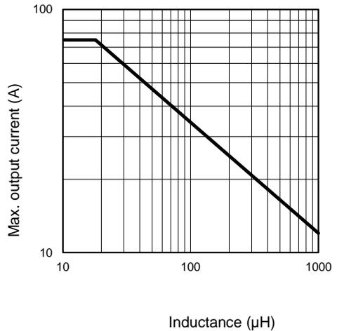
**Figure 13 – Max. iout (A) Vs inductance (μH)**
