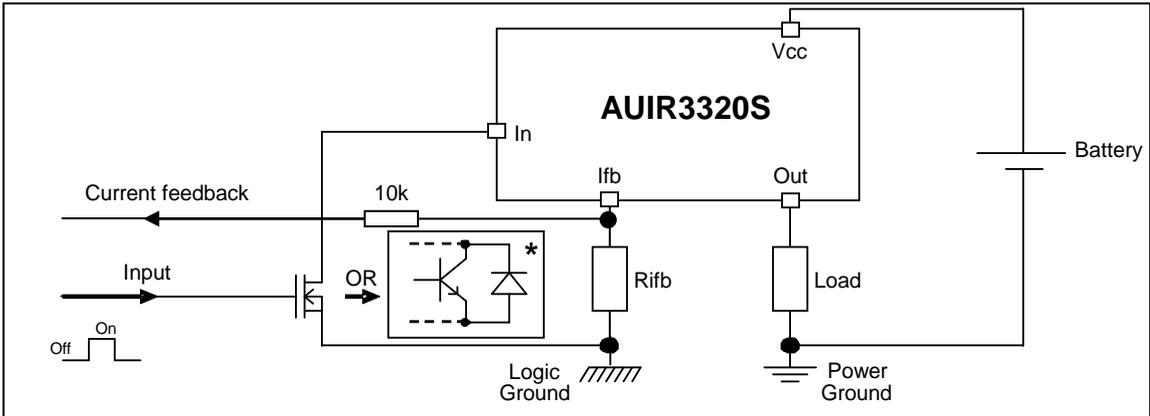
\*The diode between the collector and the emitter is necessary for the reverse battery protection
