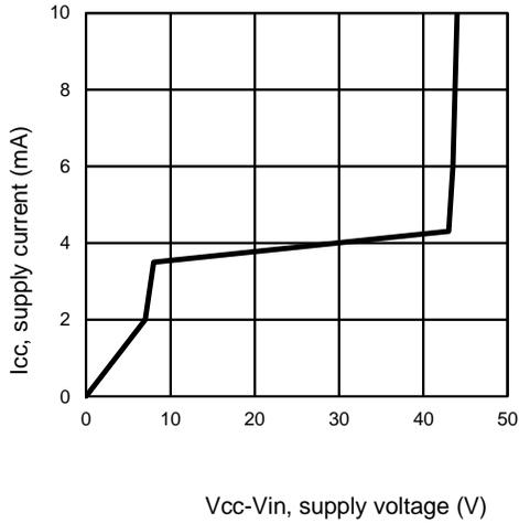
**Figure 6 – Icc (mA) Vs Vcc-Vin (V)**
