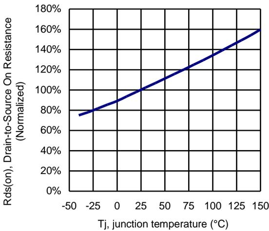
**Figure 8 - Normalized Rds(on) (%) Vs Tj (°C)**
