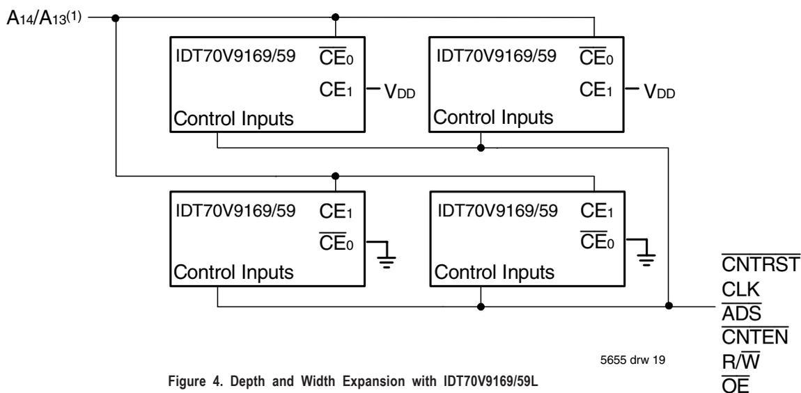
Figure 4. Depth and Width Expansion with IDT70V9169/59L
