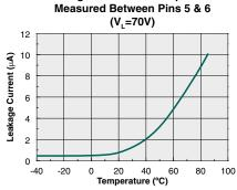
Leakage Current vs. Temperature
