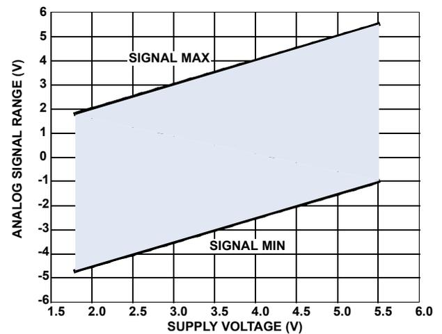
FIGURE 14. ANALOG SIGNAL RANGE vs SUPPLY VOLTAGE
