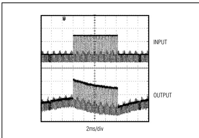
Figure 1. AC-Coupled Output
