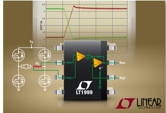
The LT1999 accurately measures fast switching currents in H-bridge motor controls, switching power supplies, solenoids and battery chargers. It features a -5V to 80V input common mode voltage range, 2MHz bandwidth, less than 1.5mV offset voltage and 0.5% gain error over temperature. With more than 80dB common mode rejection at 100kHz, the LT1999 maintains outstanding accuracy even in the presence of large square wave input voltages.
